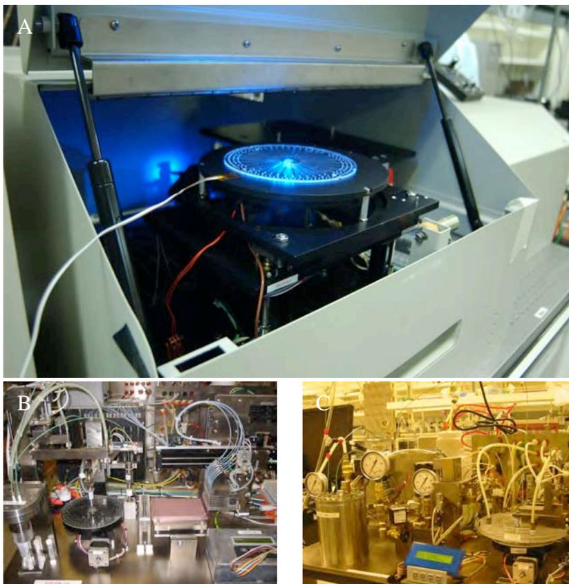
**Figure 2.** Pictures of the MCP system at VDFS consisting of (A) a four-color confocal scanner, (B) a gels/sample loader and (C) a microchip washing station.
