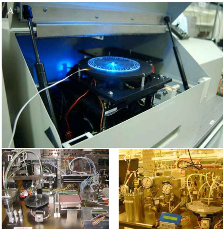
**Figure 2.** Pictures of the MCP system installed at VDFS consisting of (A) a four-color confocal scanner, (B) a gels/sample loader and (C) a microchip washing station.
