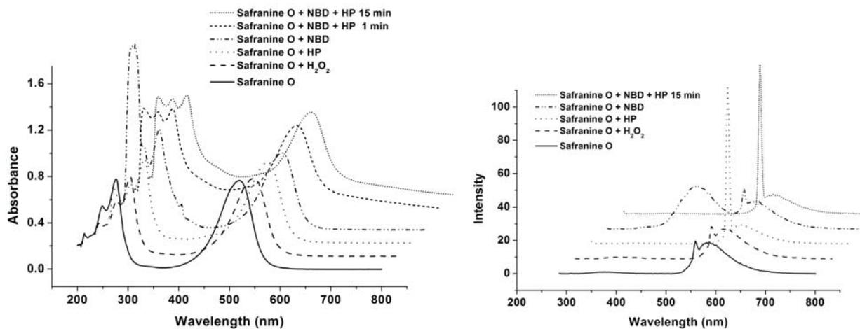
**Figure 6.** UV-Vis and Fluorescence spectra for reaction of Safranine O 2 with NBD, exc 280 nm.
