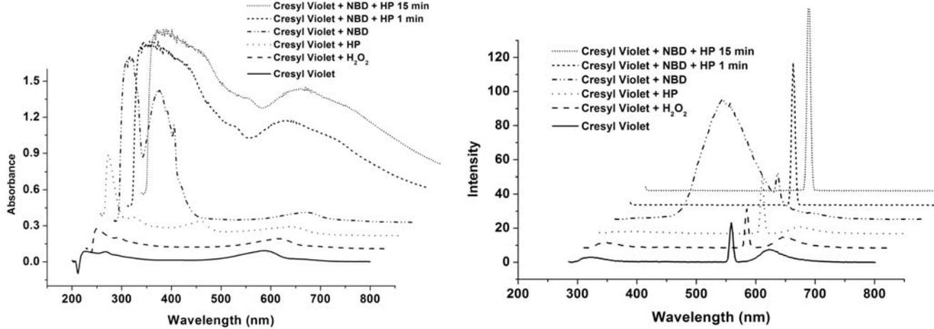
Figure 26. UV-Vis and Fluorescence spectra for reaction of Cresyl Violet 4 with NBD, exc 280 nm.
