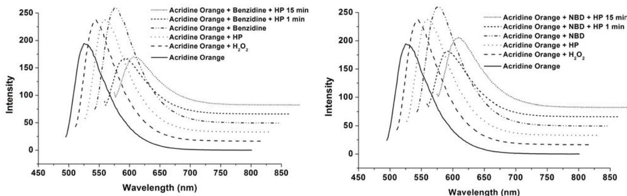
**Figure 22.** Fluorescence spectra for reaction of Acridine Orange **7** with DAB and NBD, exc 490 nm.
