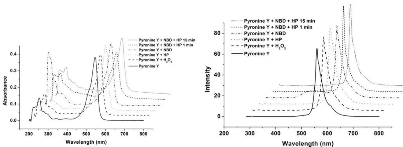
**Figure 14.** UV-Vis and Fluorescence spectra for reaction of Pyronin Y with NBD, exc 280 nm.
