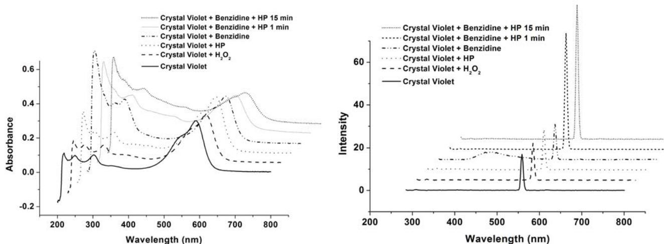
**Figure 9.** UV-Vis and Fluorescence spectra for reaction of Crystal Violet 7 with DAB, exc 280 nm.
