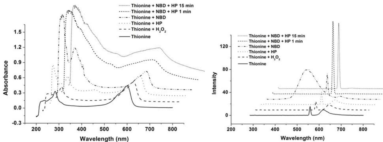
Figure 16. UV-Vis and Fluorescence spectra for reaction of Thionine 6 with NBD, exc 280 nm.
