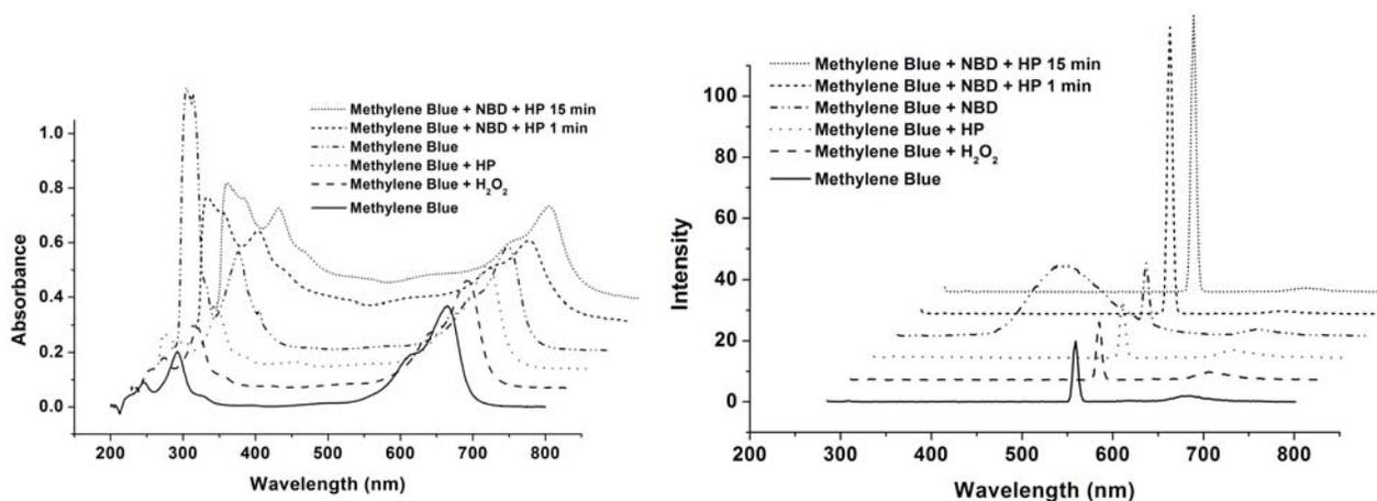
**Figure 32.** UV-Vis and Fluorescence spectra for reaction of Methylene Blue **11** with NBD, exc 280 nm.
