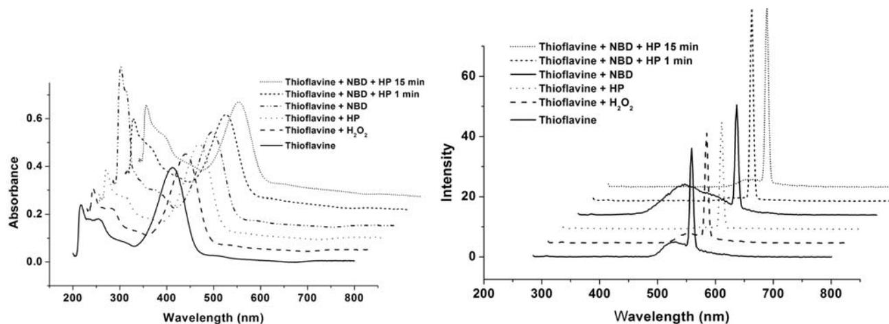
**Figure 30.** UV-Vis and Fluorescence spectra for reaction of Thioflavine T 8 with NBD, exc 280 nm.
