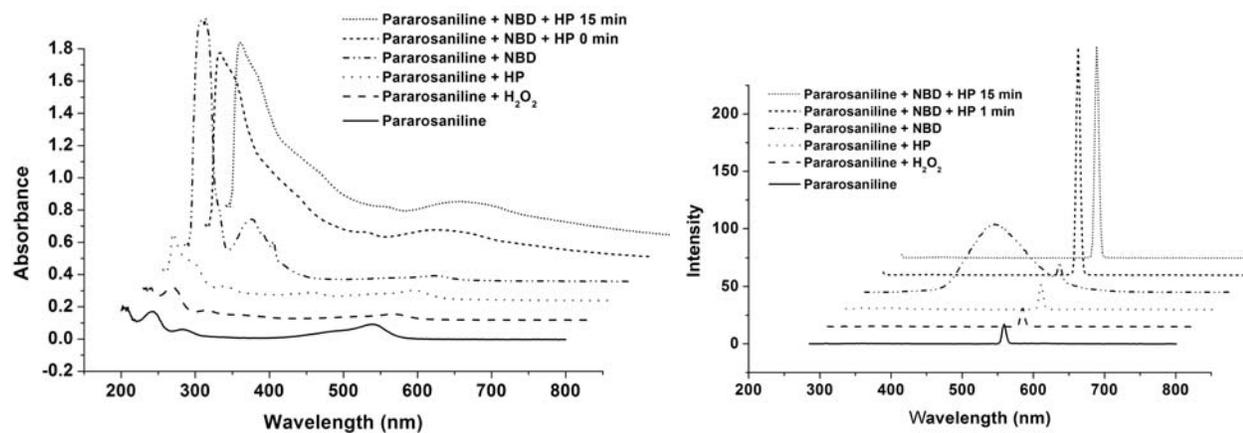
**Figure 4.** UV-Vis and Fluorescence spectra for reaction of Pararosaniline 1 with NBD, exc 280 nm.
