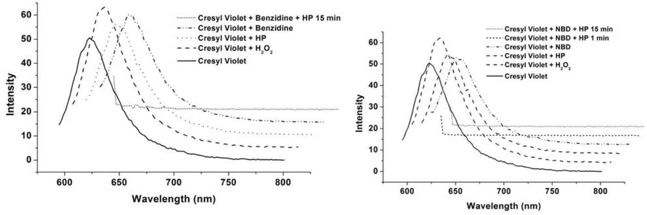
Figure 25. Fluorescence spectra for reaction of Cresyl Violet 4 with DAB and NBD, exc. 590 nm.
