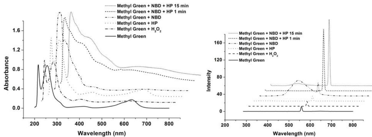
**Figure 12.** UV-Vis and Fluorescence spectra for reaction of Methyl Green **9** with NBD, exc 280 nm.
