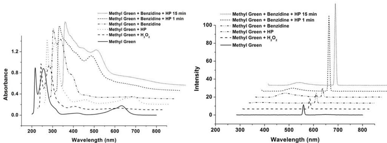
**Figure 11.** UV-Vis and Fluorescence spectra for reaction of Methyl Green **9** with DAB, exc 280 nm.
