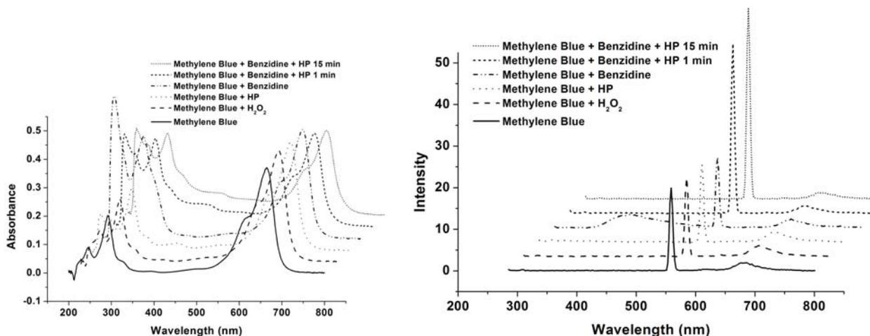
**Figure 31.** UV-Vis and Fluorescence spectra for reaction of Methylene Blue **11** with DAB, exc 280 nm.
