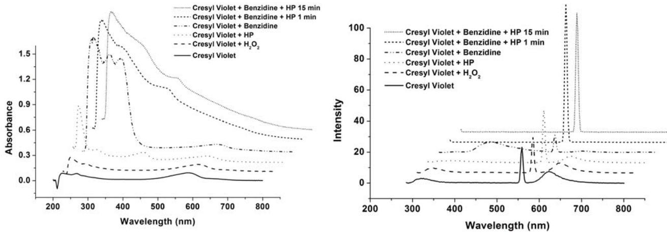
Figure 24. UV-Vis and Fluorescence spectra for reaction of Cresyl Violet 4 with DAB, exc.280 nm.
