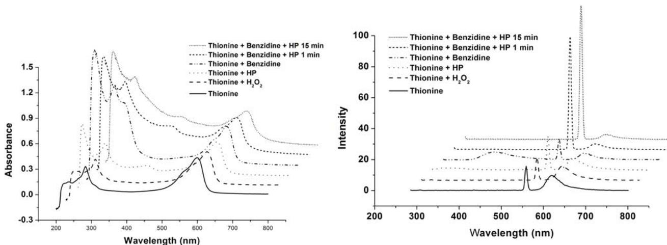
Figure 15. UV-Vis and Fluorescence spectra for reaction of Thionine 6 with NBD, exc 280 nm.
