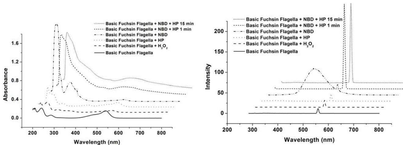
**Figure 8.** UV-Vis and Fluorescence spectra for reaction of Fuchsin Basic Flagella **3** with NBD, exc 280 nm.
