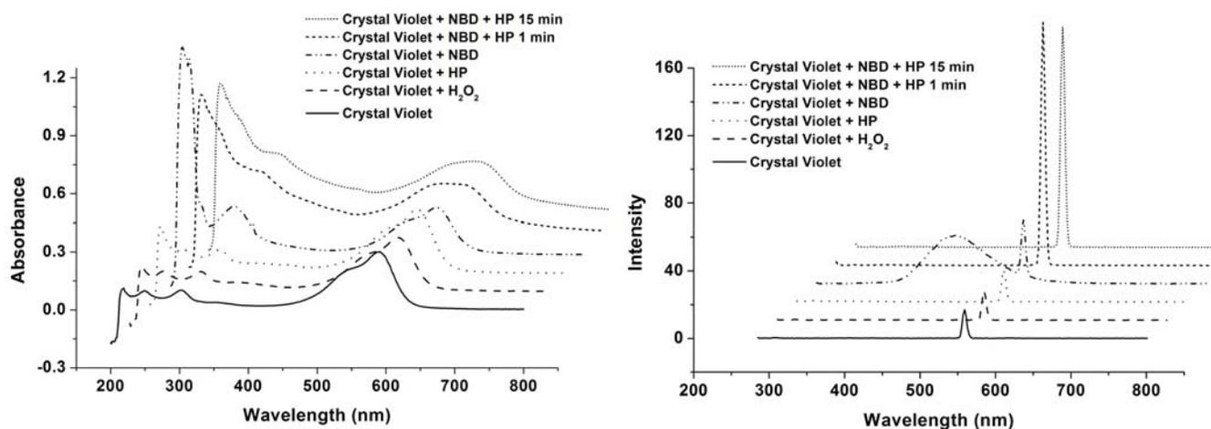
**Figure 10.** UV-Vis and Fluorescence spectra for reaction of Crystal Violet 7 with NBD, exc 280 nm.
