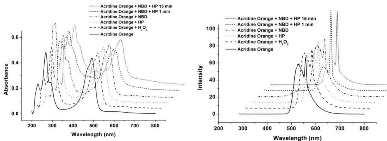
**Figure 23.** UV-Vis and Fluorescence spectra for reaction of Acridine Orange **7** with NBD, exc 280 nm.
