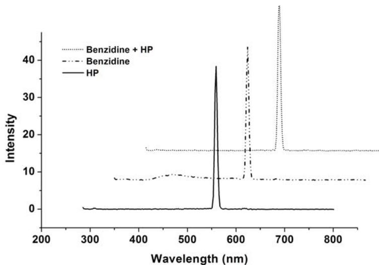
**Figure 1.** Fluorescence spectra for reaction of DAB, **14** with HP EC 1.11.1.7, exc 280 nm.
