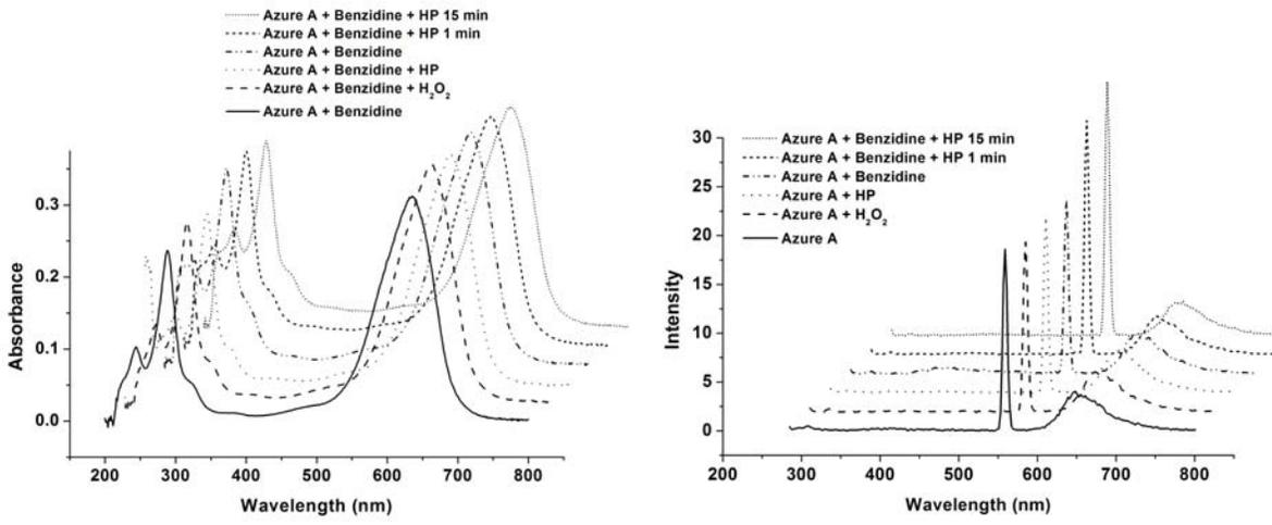
Figure 19. UV-Vis and Fluorescence spectra for reaction of Azure A with NBD, exc 280 nm.
