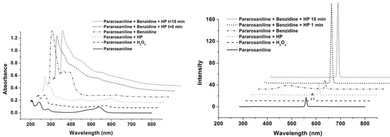
**Figure 3.** UV-Vis and Fluorescence spectra for reaction of Pararosaniline 1 with DAB, exc 280 nm.
