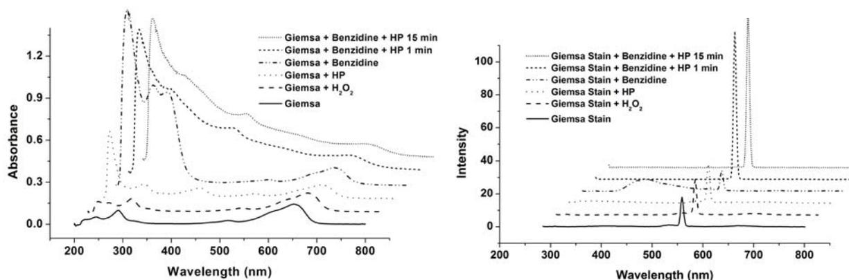
**Figure 27.** UV-Vis and Fluorescence spectra for reaction of Giemsa Stain with DAB, exc 280 nm.
