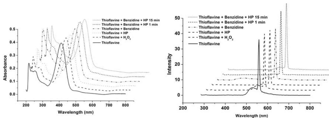
**Figure 29.** UV-Vis and Fluorescence spectra for reaction of Thioflavine T 8 with DAB, exc 280 nm.
