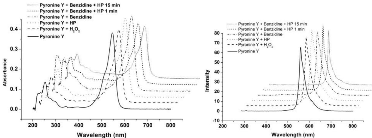
**Figure 13.** UV-Vis and Fluorescence spectra for reaction of Pyronin Y with DAB, exc 280 nm.
