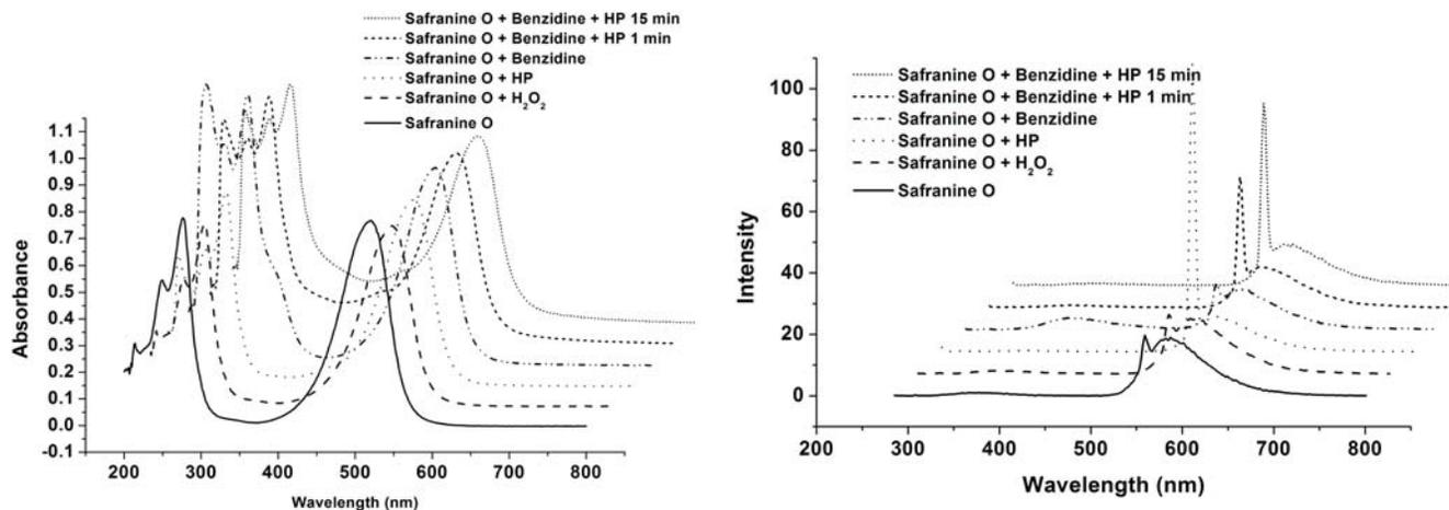
**Figure 5.** UV-Vis and Fluorescence spectra for reaction of Safranine O 2 with DAB, exc 280 nm.
