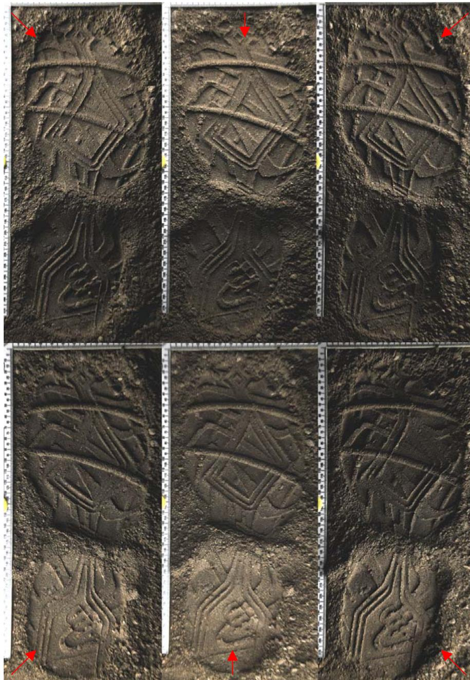
Exhibit 1: The red arrows depict six of the infinite light positions from a PTM image. An infinite number of light positions can be viewed with this technique using the same interactive image.
