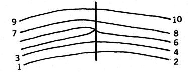
Figure 3. 'Offsetting' of generating lines.
