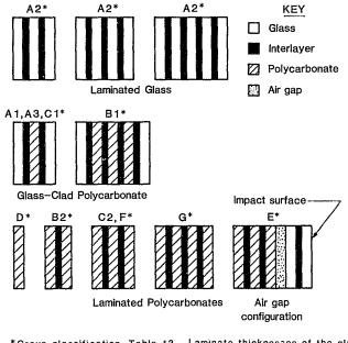
\*Group classification, Table 13. Laminate thicknesses of the glass, polycarbonate, and interlayer varied – see Tables 3,4, & 5. NOTE: Laminate thickness not drawn to scale.
