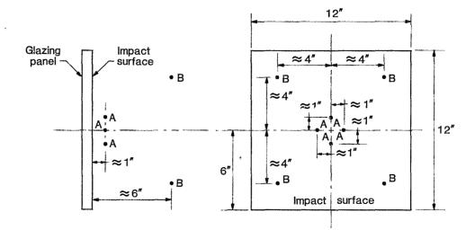
FIGURE 11. Locations where hot-wire anemometer readings were taken. Hot-wire anemometer tip was rotated at each of the eight locations and the maximum reading obtained at each location was recorded.
