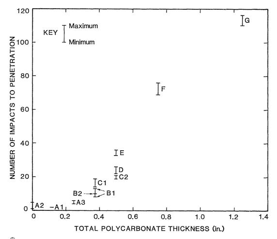
**PIGURE 14.** Number of impacts to penetration versus total polycarbonate thickness (thickness of polycarbonate laminates taken collectively)—see table 13 for definition of groups A1,A2,...F,G, and the number of panels in each group.
