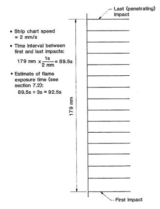
FIGURE 13. Sample strip chart recorder output showing the time history of the 16 impacts required for penutration. The time interval between the first and last impacts and an estimate of the flame exposure time are also shown.
