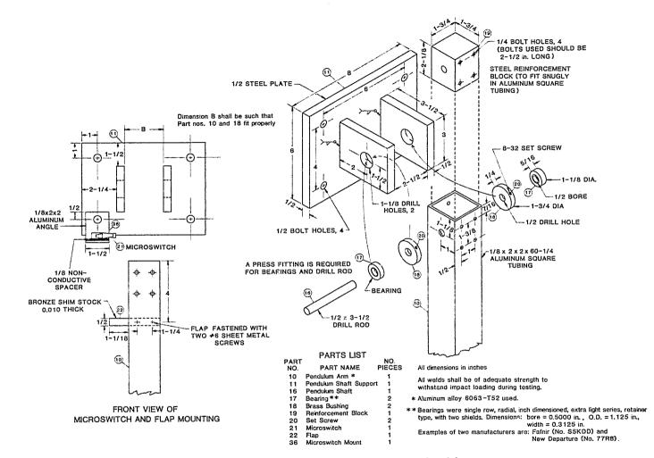
FIGURE A2. Pendulum support system and upper section of pendulum arm.
