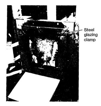
FIGURE 9. Steel glazing frame, nonimpact side. Test panel no. 69, which had been tested, was secured to the glazing frame by the steel glazing clamp with bolts as shown.
