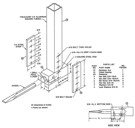
FIGURE A3. Chisel housing assembly.
