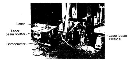
FIGURE 8a. Velocity measuring apparatus, including laser, laser beam splitter, laser beam sensors, and chronometer.
