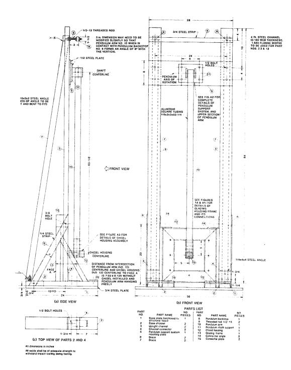
FIGURE A1. Pendulum apparatus.
