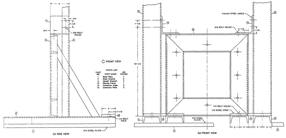
FIGURE A5. Connection details for glazing frame.
