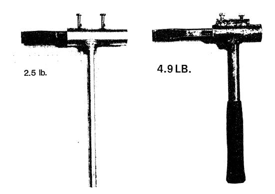
FIGURE 1. Hand-held hammers, weighing 2.5 and 4.9 lb, used for human swings to determine an impact damage level. Hammer head secured a 1-in steel chisel weighing 1.3 lb. (The 2.5 and 4.9 lb hammer weights include the weight of the 1.3 lb chisel).
