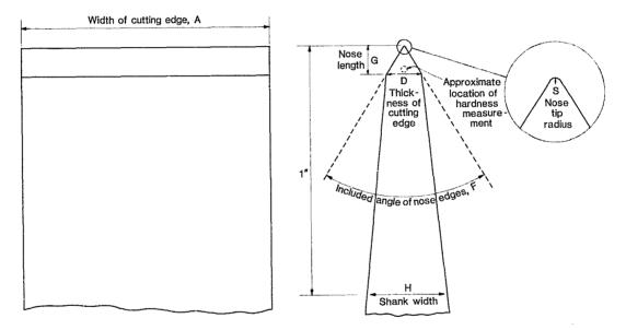
FIGURE 10. Chisel geometrical nose variables measured. The approximate location of the hardness measurement is also shown.
