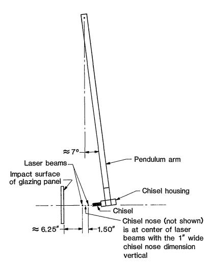
FIGURE 8b. Position of pendulum, chisel nose, and laser beams when chisel velocity was measured.
