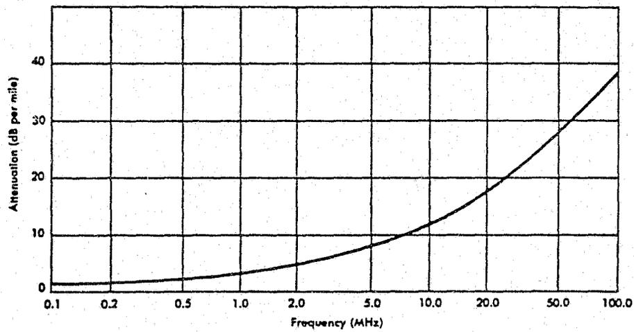
Figure 3.9 Attenuation Rate Versus Frequency for  $\emptyset$ .375 in. dia., 75 Ohm Broadband Coaxial Cable
