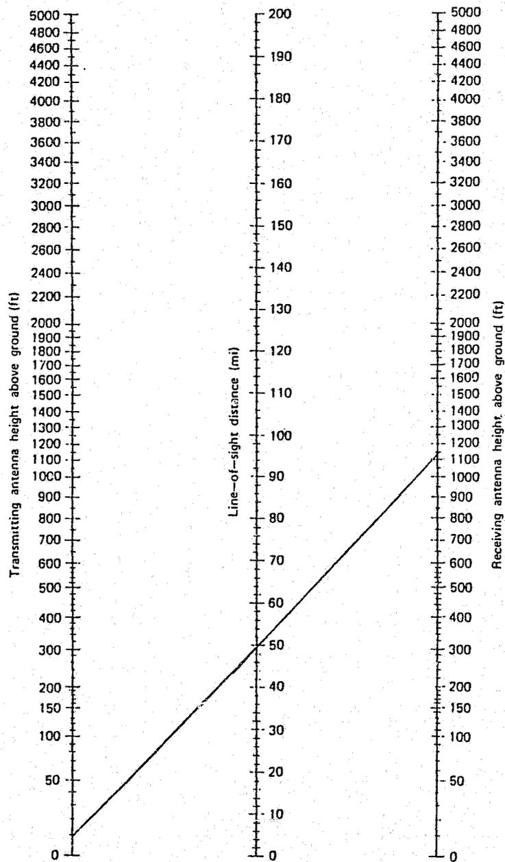
Figure 3.11 Line of Sight Propagation Distances for a Smooth Spherical Earth with  $K = 1.33$
