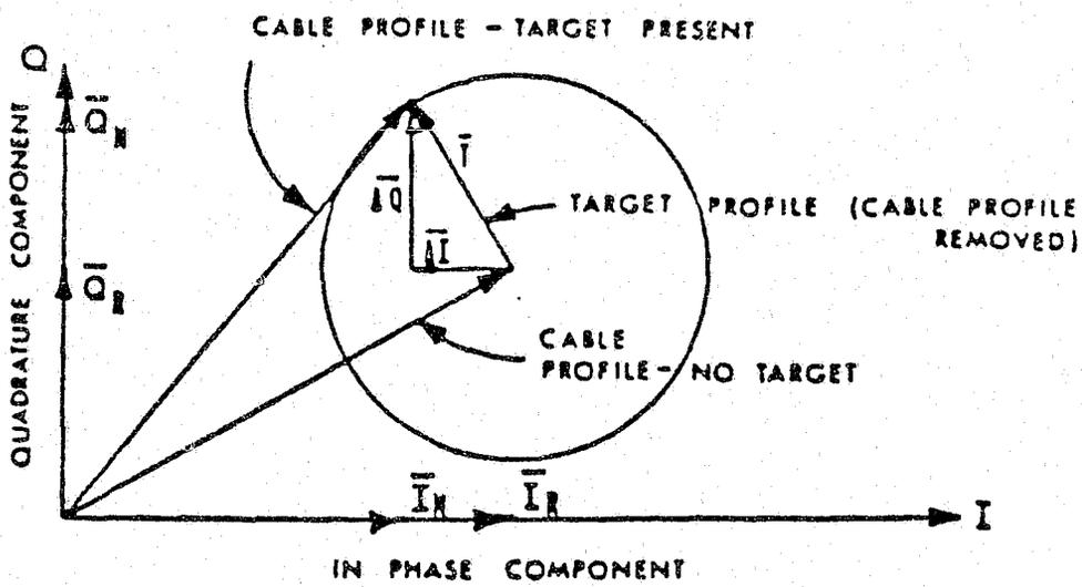
Figure 2.5 Vector Subtraction of the Inphase and Quadrature Phase Components to Determine the Target Profile
