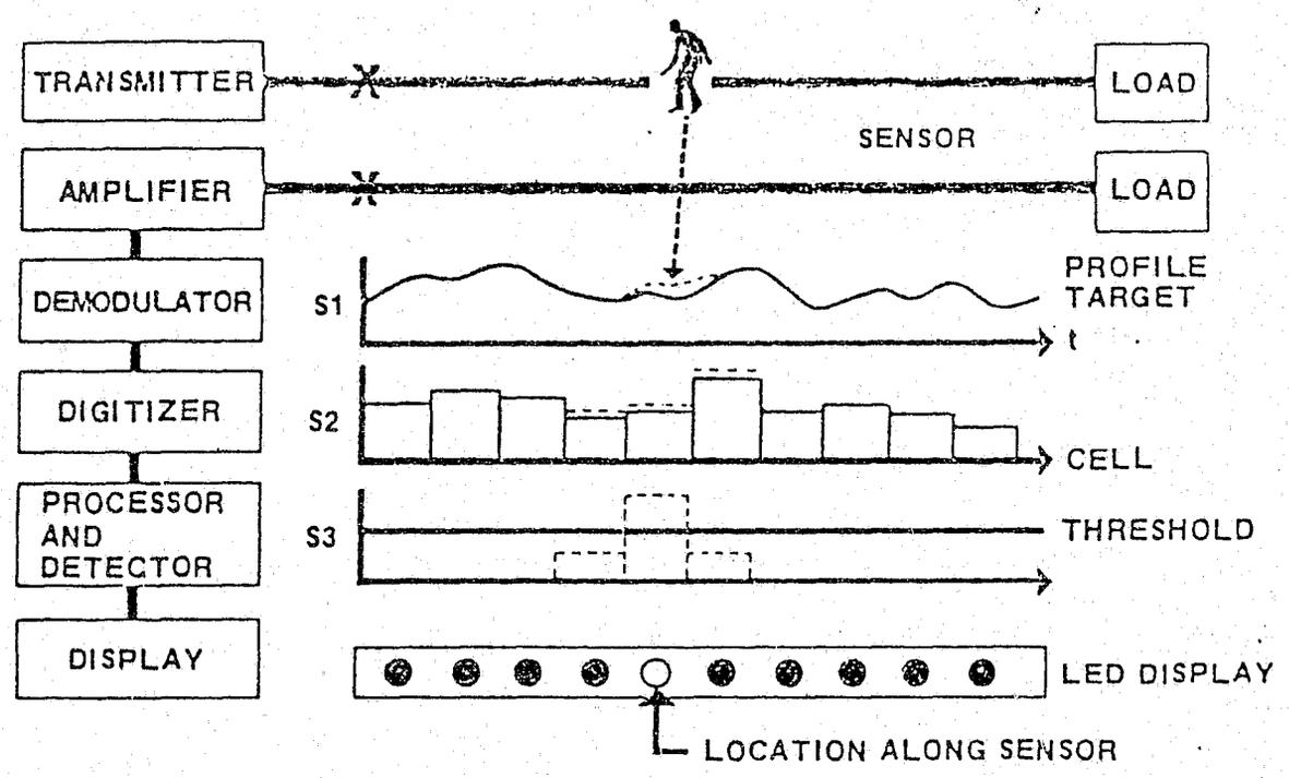
Figure 2.1 Operation of the GUIDAR PCCS System
