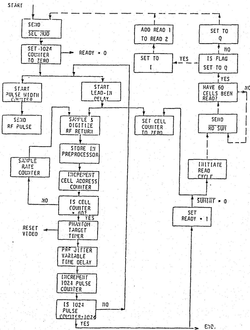
Figure 2.4 GUIDAR Signal Processing Flow Chart
