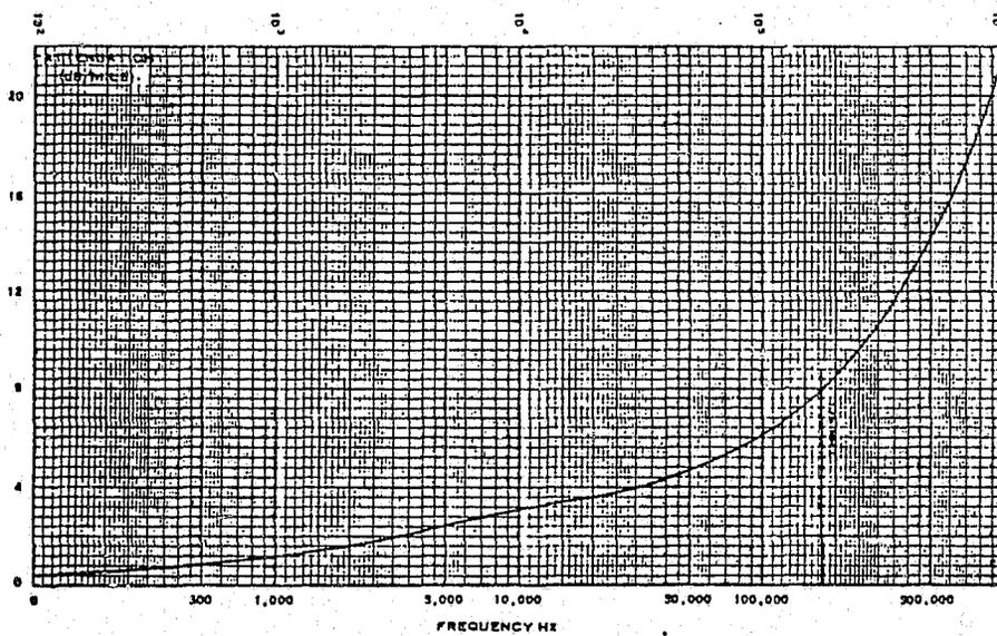
Figure 3.4 Attenuation Versus Frequency for a Typical 19 AWG Twisted Wire Pair Cable
