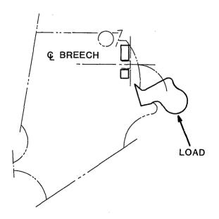
FIGURE 7. Hammer test setup.
