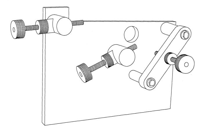
FIGURE B-1. Sketch of headspace test fixture.
