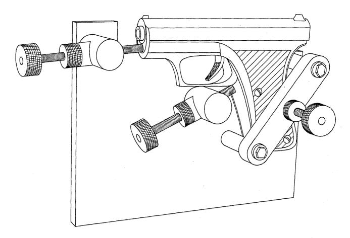
FIGURE B-2. Sketch of headspace test fixture with pistol in place for headspace measurement.
