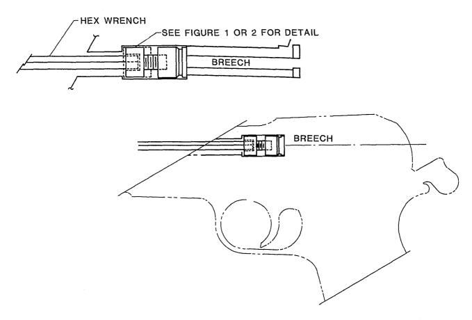
FIGURE 5. Headspace gage usage.
