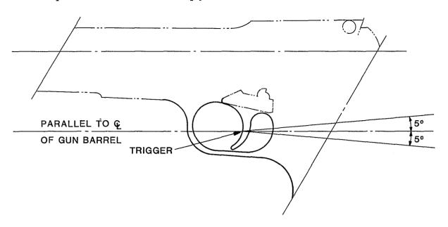
FIGURE 6. Trigger pull test setup.
