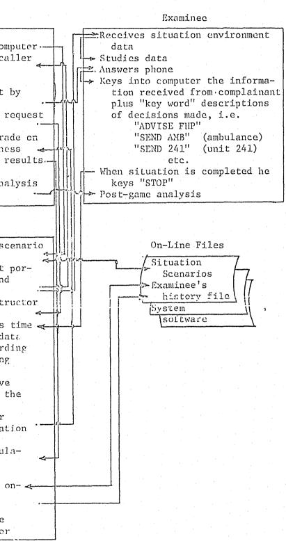
Figure 20 The Figure Above Shows the Logic Flow of the Computer Augmented Game Model
