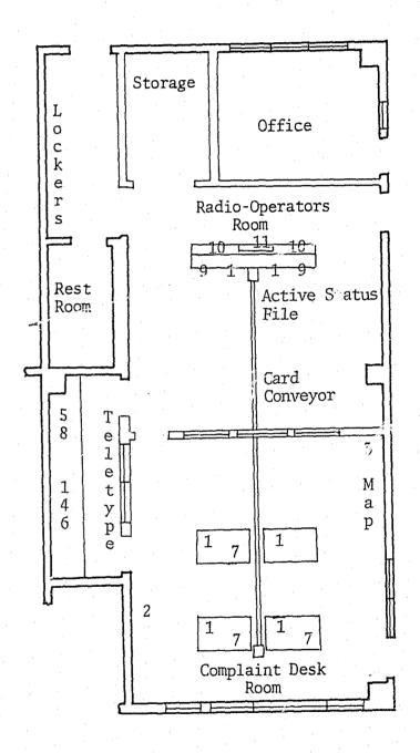
Figure 9 Showing Major Equipment Locations For Each Specialized Task Of Command And Control.
