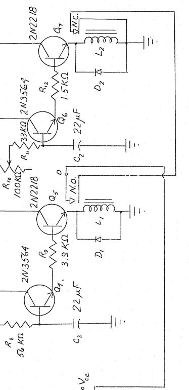
Figure 60: Solenoid Control Timing Circuitry
