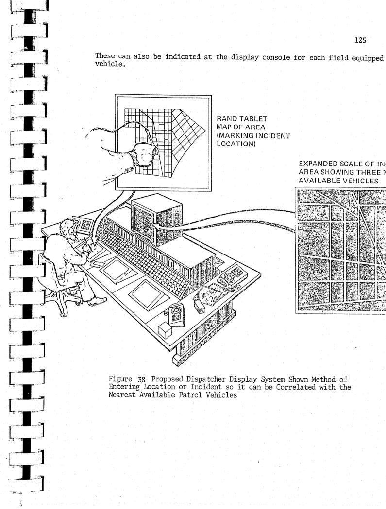
RAND TABLET MAP OF AREA (MARKING INCIDENT LOCATION) EXPANDED SCALE OF INCIDENT AREA SHOWING THREE NEAREST AVAILABLE VEHICLES
