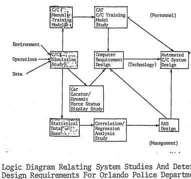
Figure 2: Logic Diagram Relating System Studies And Determination Of Design Requirements For Orlando Police Department Automated Command/Control System Identifies Three Major Areas Of Effort, Personnel, Technology and Management, Which Are Required.
