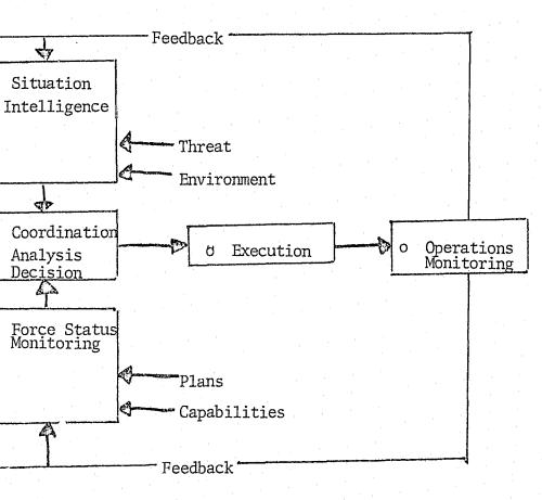
Figure 1 : Functional Block Diagram Of Basic Command/Control Process Shows Its Dependency On A Closed Loop Feedback System.
