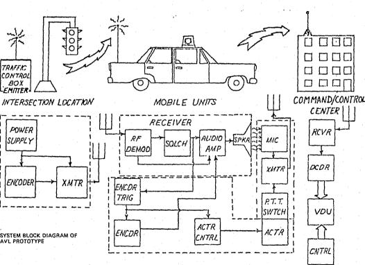
Figure 17 Block Diagram of the System
