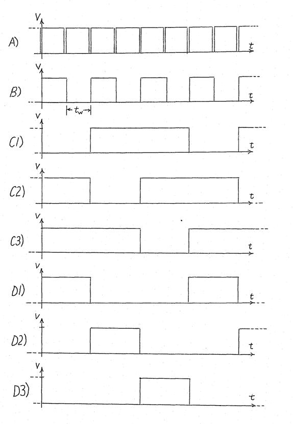
Figure 57: Pulse Trains: A) N74123 output, B) clock waveform, C) decoder/demultiplexer enabling waveforms, D) decoder/driver blanking waveforms.
