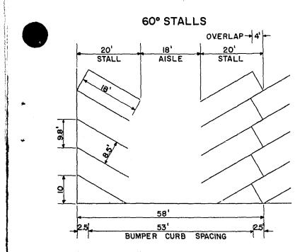
Figure 13-7. Minimum dimensions for parking area layout, 60° stalls.
