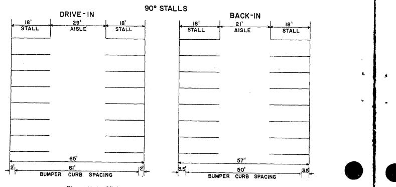
Figure 13-6. Minimum dimensions for parking area layout, 90° stalls.
