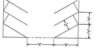
Figure 13-5. Dimensions for parking stalls for various types of parking.
