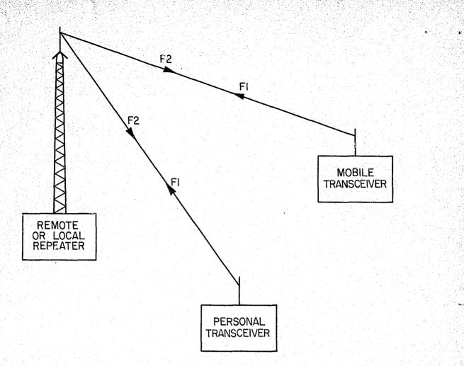
Figure 3-Block Diagram of a Repeater Using Single Antenna and Duplexer
