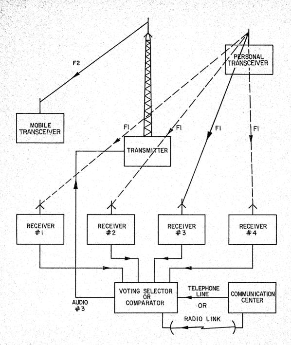
Figure 5-Block Diagram of a Repeater Using Voting Receivers
