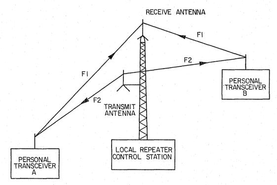
Figure 1-Block Diagram of a Repeater Under Local Control
