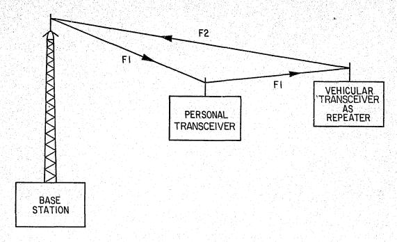
Figure 6-Block Diagram of a System Using the Vehicular Transceiver as a Repeater
