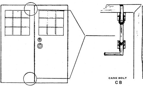
Many homes with pairs of doors, use half-barrel slidebolts on the inactive door. These are weak and inadequate.
