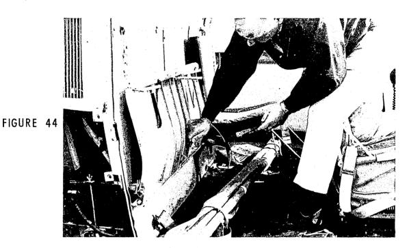
Upon landing at an accident, the trooper attends to the injured persons while the pilot readies the cabin for the litter as shown in Figure 44. It is necessary to open the lock which secures the drop seat leg to the floor, using a screwdriver (½ twist). The seat is then raised and secured to the rear bulkhead using a hookeye.
