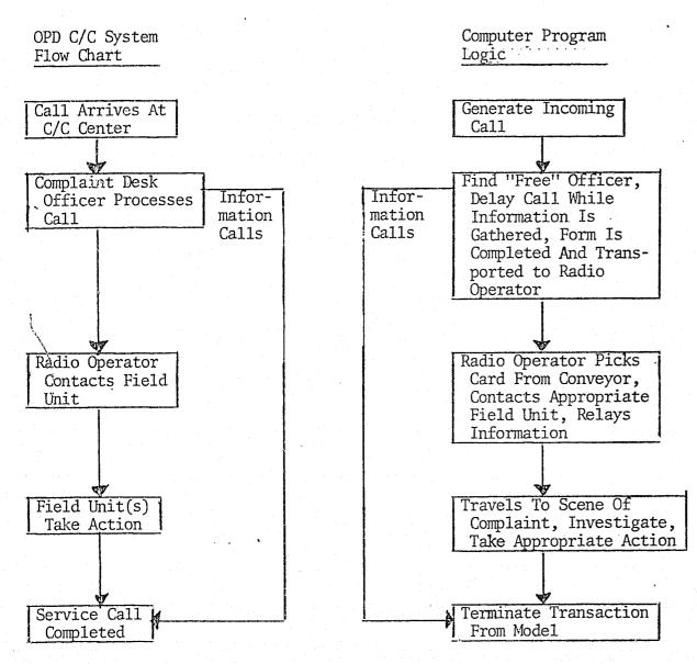
Figure 2. The comparison of GPSS/360 Program Logic Blocks to Flow Chart of actual system.
