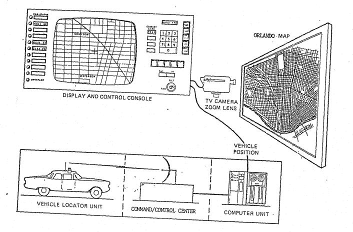
Figure 6: FLAIR System Concept Shows Major Functional Components and their Interrelationship
