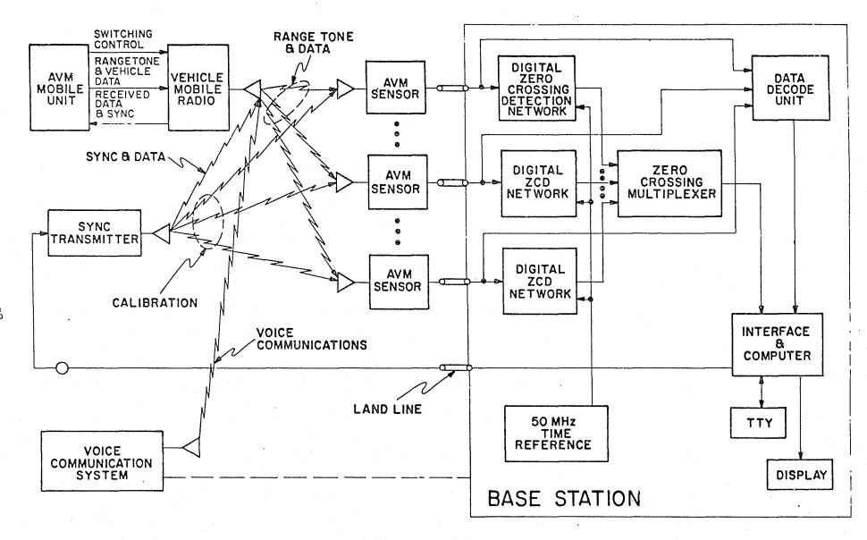
Figure 2. Simplified AVM System Block Diagram
