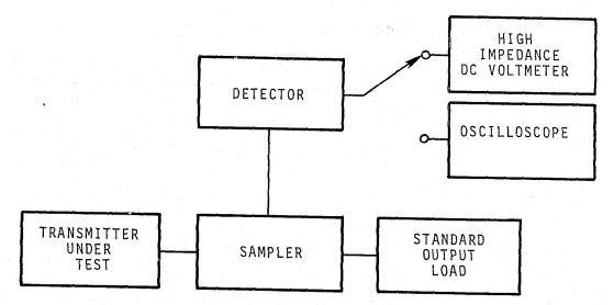
FIGURE 4. Block diagram for AM hum and noise measurement.
