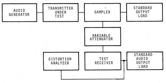
FIGURE 6. Block diagram for harmonic distortion and FM hum and noise measurements.
