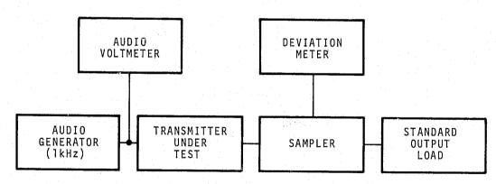
FIGURE 8. Block diagram for frequency deviation and modulation limiting measurements.
