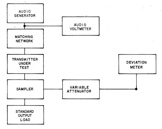
FIGURE 7. Block diagram for audiofrequency response measurement.
