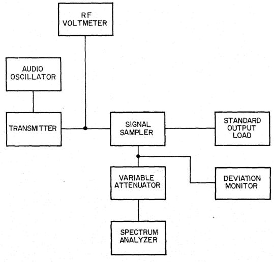
FIGURE 12. Block diagram for sideband spectrum measurement.
