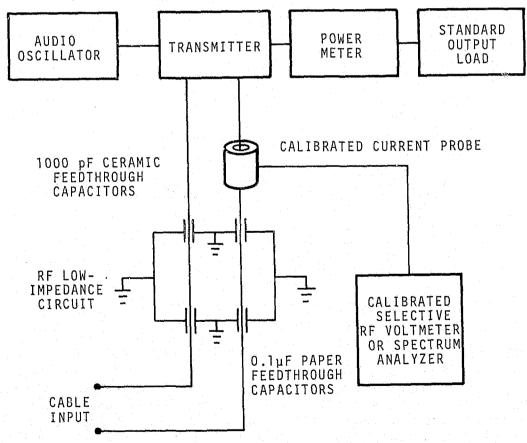
FIGURE 10. Block diagram for conducted spurious emissions measurements on cables.
