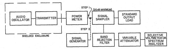
FIGURE 9. Block diagram for conducted spurious emissions at the antenna terminals.
