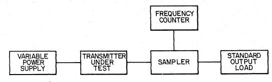
FIGURE 3. Block diagram for frequency stability measurement.
