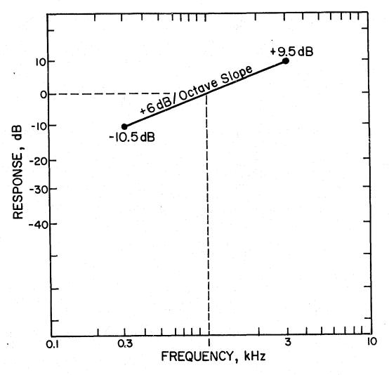
FIGURE 1. Audiofrequency response characteristics of fixed and base station FM transmitters.
