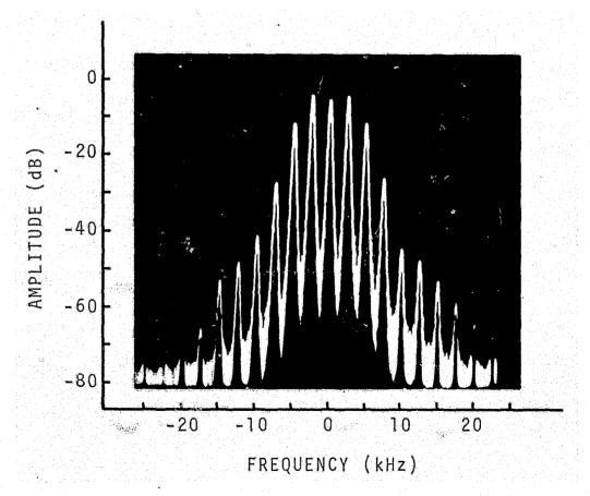
FIGURE 13. Typical sideband spectrum on a tube-type transmitter using a 2.5 kHz tone 16 dB greater than that required to produce  $\pm$  2.5 kHz deviation at 1.0 kHz.
