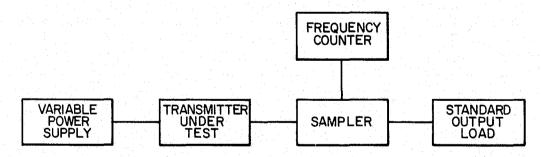
FIGURE 3. Block diagram for frequency stability measurement.
