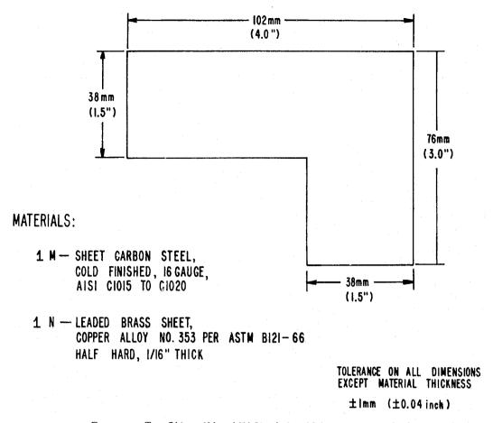
FIGURE 2. Test Objects IM and IN Simulating .25 Semiautomatic Pistol
