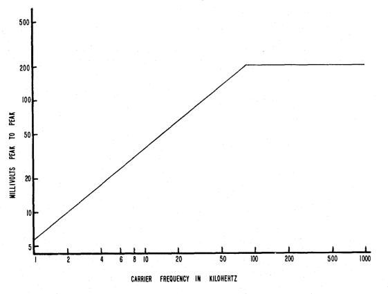
FIGURE 1. Maximum Induced Voltage in 22.5cm Loop at 2.5cm Separation Distance
