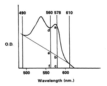
Figure 9.1 Scheme for Determination of α- ratio (after Kind et al., 1972)
