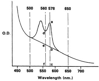
Figure 9.2 Scheme for Determination of  $\infty$ s - ratio (after Kind and Watson, 1973)
