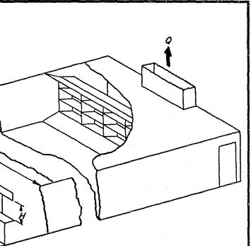
Maximum grille velocity = 400 fpm Size for uniform distribution Bureau of Mines approved lead dust respirator is Acoustical material on walls, ceiling and thick fabric on bench top are recommended AMERICAN CONFERENCE OF GOVERNMENTAL INDUSTRIAL HYGIENISTS INDOOR PISTOL AND SMALL BORE RIFLE RANGE VENTILATION
