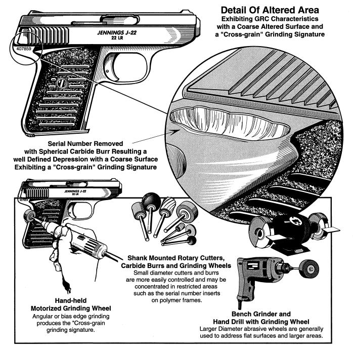
Abrasive Grinding Devices used in Serial Number Removal that produce the GRC characteristics
