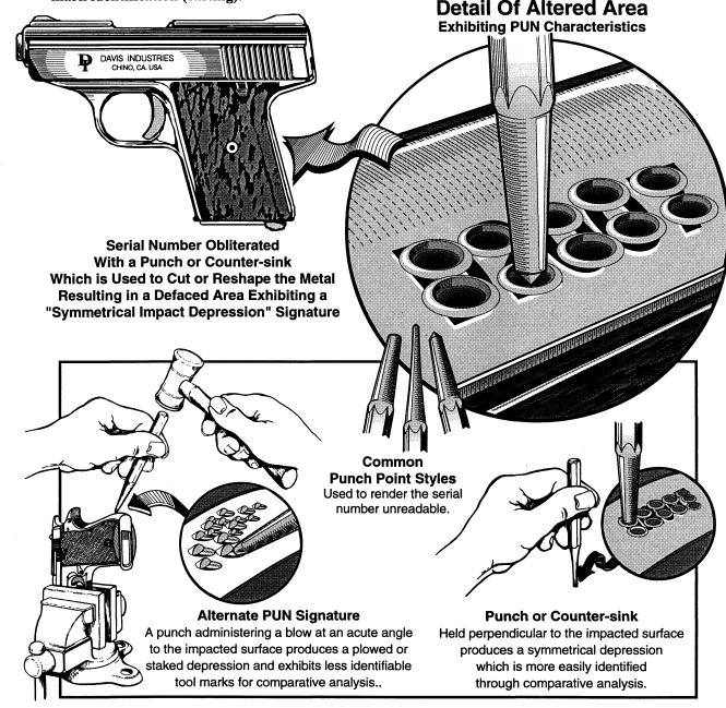
Compression Devices used in Serial Number Removal that produce the PUN characteristics
