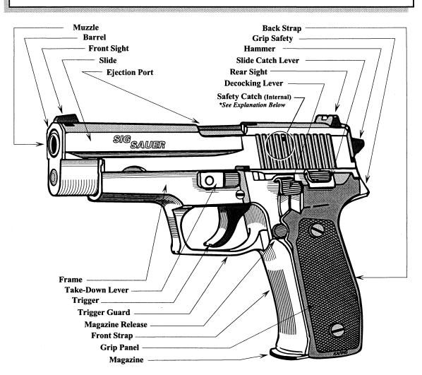
\* The Safety Catch is an internal design and locks the firing pin until the trigger is intentionally pulled which automatically releases the safety mechanism to initiate the firing sequence.
