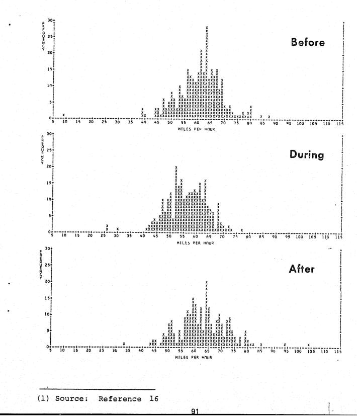
FIGURE 4-16: Distributions of Spot Speeds for Same- and Opposite-Sides of Road Combined, Before, During and After, Adjacent Application of An "Arrest" Stationary Enforcement<sup>(1)</sup>
