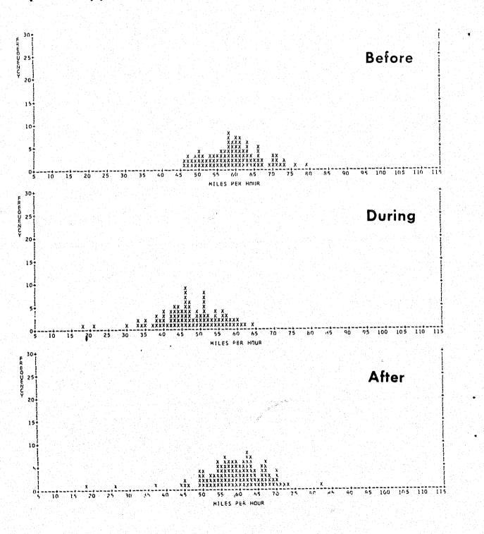
It was noted in the previous study that it was not possible to implement a planned effort to estimate the affects of more conventional enforcement techniques on traffic flow variables because data collection problems brought on by repairs on the test highway. In the present study, the short-term effects of a concentrated warning-citation program in the vicinity of a CHTIS sensor site were measured.
