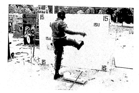
Figure 139. Test 15U. Kicking Out Plasterboard
