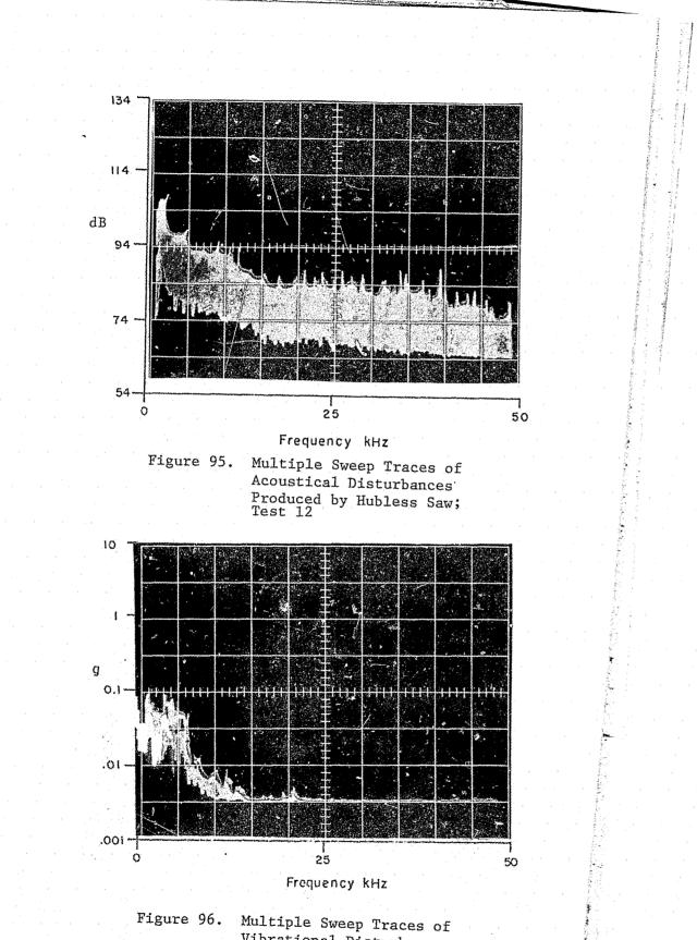
Multiple Sweep Traces of Vibrational Disturbances Produced by Hubless Saw; Test 12 82
