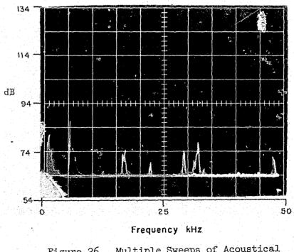
Figure 26. Multiple Sweeps of Acoustical Disturbances from Cutting Maul; Test 3A
