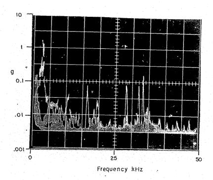
Figure 122. Test 13K. Multiple Sweep Trace of Vibrational Disturbances Resulting from Ram Attacks 99
