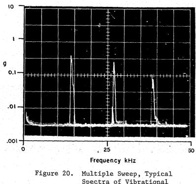
Figure 20. Multiple Sweep, Typical Spectra of Vibrational Disturbances; Test 2B
