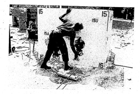
Figure 140. Test 15U. Opening Produced by Kicking Out Plasterboard
