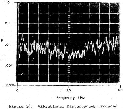
by 14" Gasoline-Powered Wheel Saw; Test 4A 35
