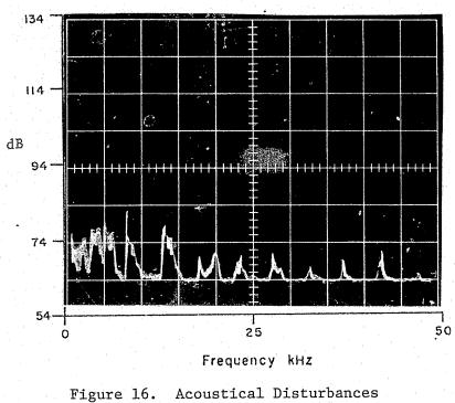
re 16. Acoustical Disturbances Resulting from Drilling; Test 2B
