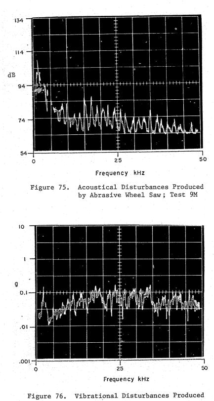
by Abrasive Wheel Saw; Test 9M
