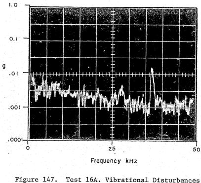
Igure 147. Test 16A. Vibrational Disturbances Produced by Torch
