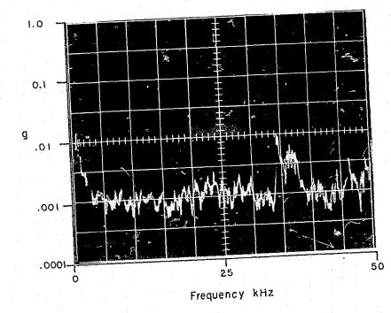
Figure 154. Single Sample of Vibrational Disturbances Produced by Second Burning; Test 16U 122 6. DISCUSSION OF BARRIER PANEL TEST RESULTS
