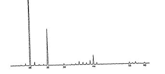
Fig. 4. Representative mass spectrum of NYCPD heroin head gases at room temperature. Some of the compounds showing detectable mass peaks are nitrogen (air) (28), methanol and ethanol (31, 45, 46), oxygen (air) (32), hydrochloric acid (36, 38), acetone (43, 58), carbon dioxide (44), and acetic acid (60).
