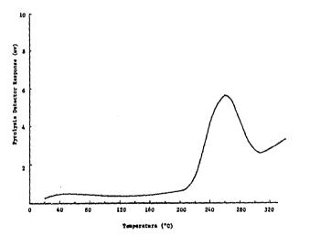
Fig. 2. Pyrolysis curve (gas-evolution rate vs temperature) from 10-mg sample of NYCPD heroin.
