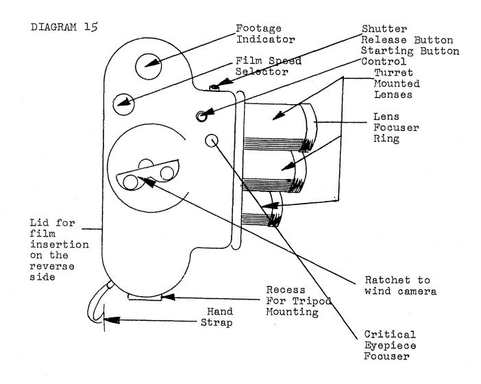
Predetermine the distance (if it is possible) the distance at which you will be photographing. 6. The camera is held firmly in both hands for ordinary film making but recommend that it be set on a tripod for
