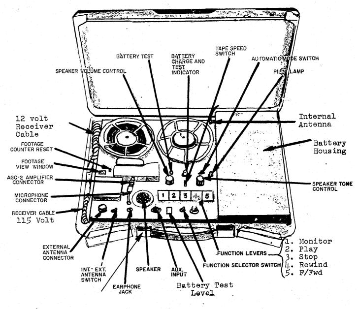
Operating the Kel Receiver 1. Power source: there are three ways in which the receiver may be operated:
