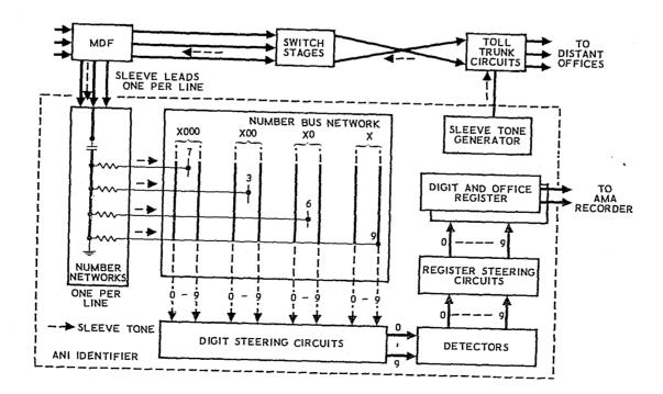
Figure 23. AMA Identifier. Typical Calling Number Identifier Circuit Used in Step-by-Step and No. 1 Crossbar Offices with AMA
