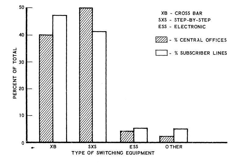
Figure 18. Distribution of Central Offices and Lines by Type of Switching Equipment - 1973
