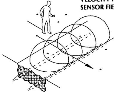
BURIED PORTED CABLE SENSOR SIZE AND SHAPE OF DETECTION PATTERN IS DEPENDANT UPON CABLE SEPARATION, BURIAL DEPTH, AND SOIL CONDUCTIVITY LEVELS.
