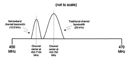
Figure 16-2: Public Safety UHF Frequency Band, 450-470 MHz
