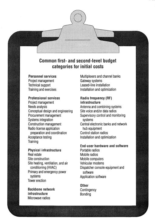
Figure 8-4: Common First- and Second-Level Budget Categories for Initial Costs
