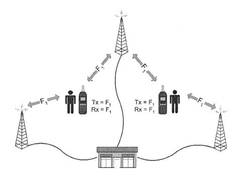
Figure 16-6: Simulcast Simplex Radio Example
