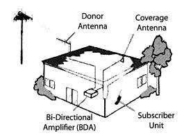
Figure 16-8: Bi-Directional Amplifier Example
