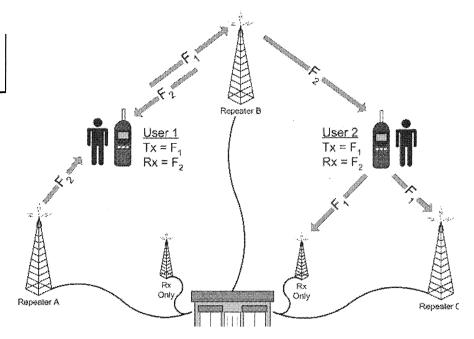
Figure 16-7: Simulcast Repeaters with Remote Receivers
