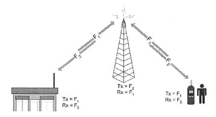
Figure 16-5: Half-duplex (Repeater) Radio Example
