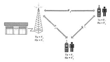
Figure 16-4: Simplex Radio Example
