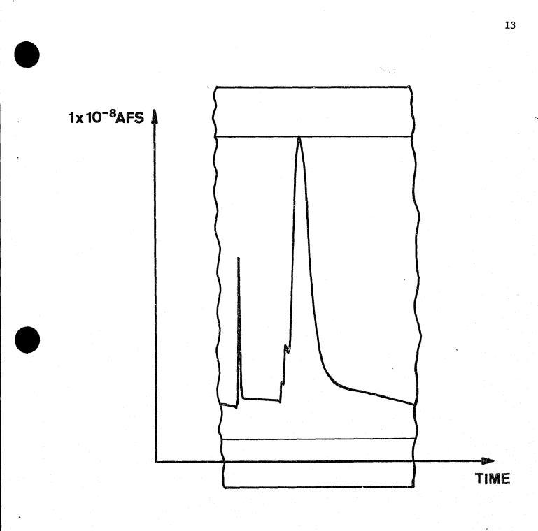
FIGURE 5. Vapor Trace Analyzer's Strip Chart Record of a TNT Detection(Before Drying TNT) at a retention time (R.T.) of approximately 9 seconds. With the sound alarm set on the 9 second peak, (assumed to be the TNT peak) two toiletries,-Mennen's Skin Bracer and Right Guard deodorant used for the interference tests produced false alarms.
