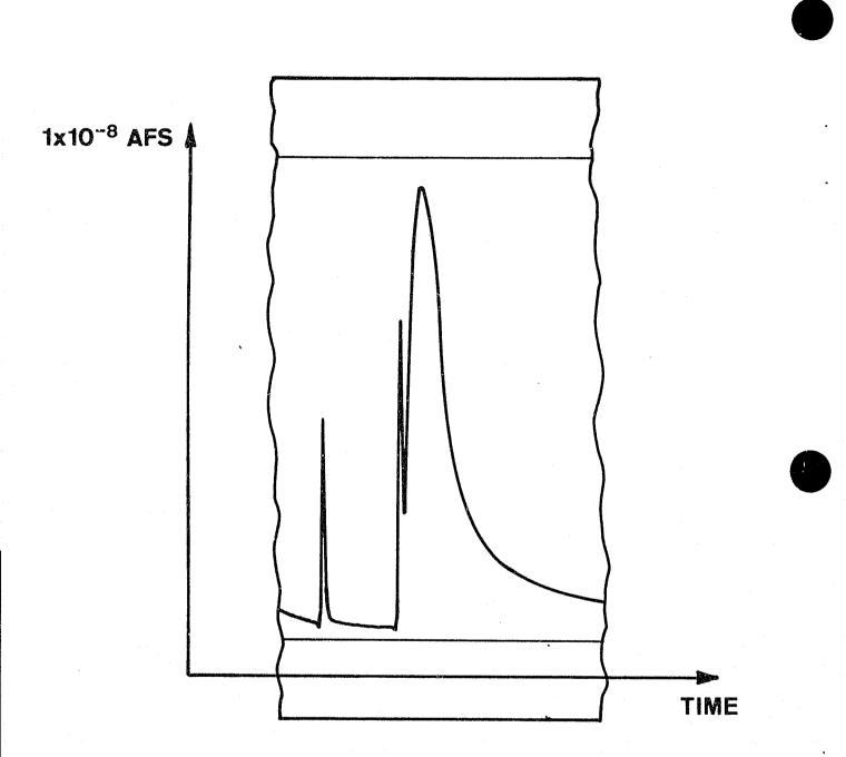
FIGURE 4. Vapor Trace Analyzer's Strip Chart Record of a Dynamite Detection
