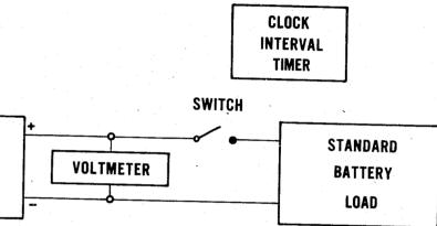
FIGURE 1. Block diagram for closed-circuit voltage test.
