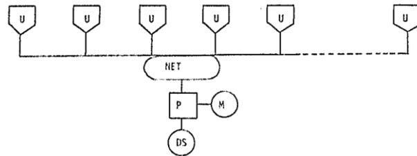
This is perhaps the simplest of CLIS configurations. All users would interface their terminals directly with a single-processor complex. This configuration also provides the greatest degree of centralized control.
