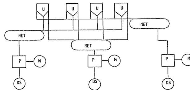
This system configuration provides for a communication network for each application area or groups of application areas. It also provides for distributed processing functions. Each user would have one or more terminals to connect to the selected application area.
