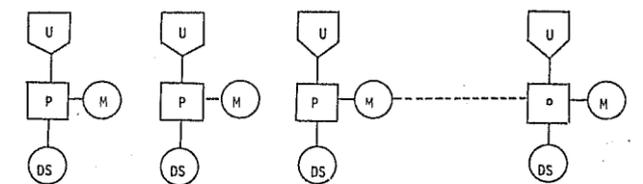
This configuration provides each user with a complete processing and data storage capability. There is no direct communication with a central system nor other laboratories.
