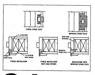
ened the door sufficiently so that a single blow will just tear the lock right out of the door.
