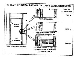
and thus, you double the resistance to the jimmying or to the spreading attack. If you pick up a couple of lousy pieces of scrap two-by-four and put them on either side of the first two entry studs, you add another four hundred pounds of spreading resistance.
