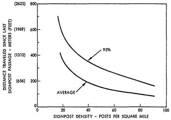
Fig. 12. Distance traveled since the previous signpost passage for a proximity system. This is equivalent to uncertainty in vehicle location which is location error. Square blocks and a density of 90 blocks per square mile were assumed for this case.
