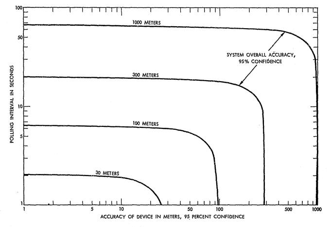
Fig. 10. AVL system accuracy
