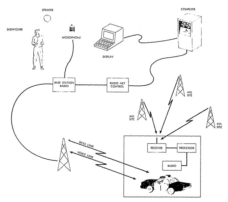
Fig. 7. Typical elements of a radiolocation AVL system
