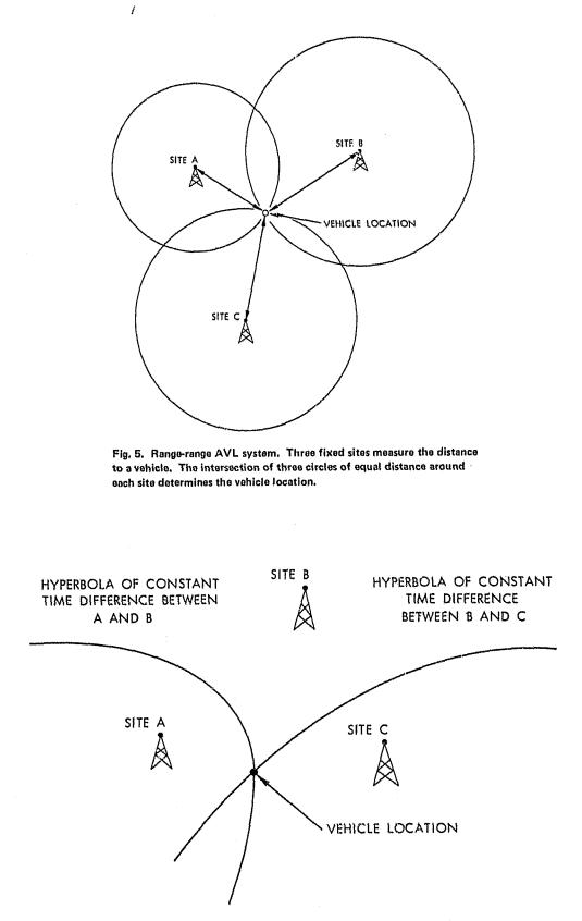
Fig. 5. Hyperbolic AVL system. Three fixed sites use the measured difference in radio signal travel time to determine the intersection of two hyperbolic curves.
