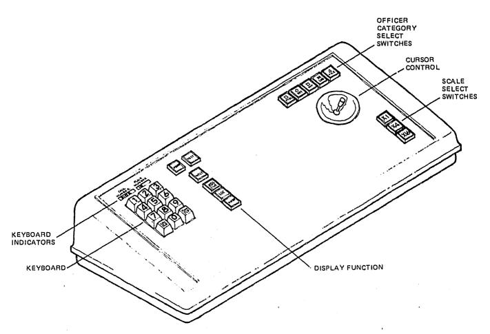
Fig. B-7, Typical dispatcher's control console
