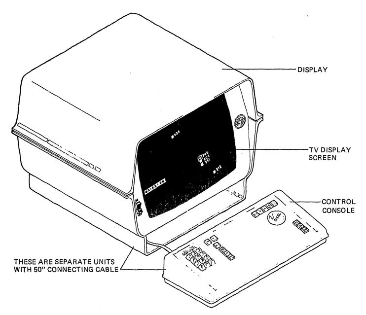
Fig. B-5. Typical control console/display
