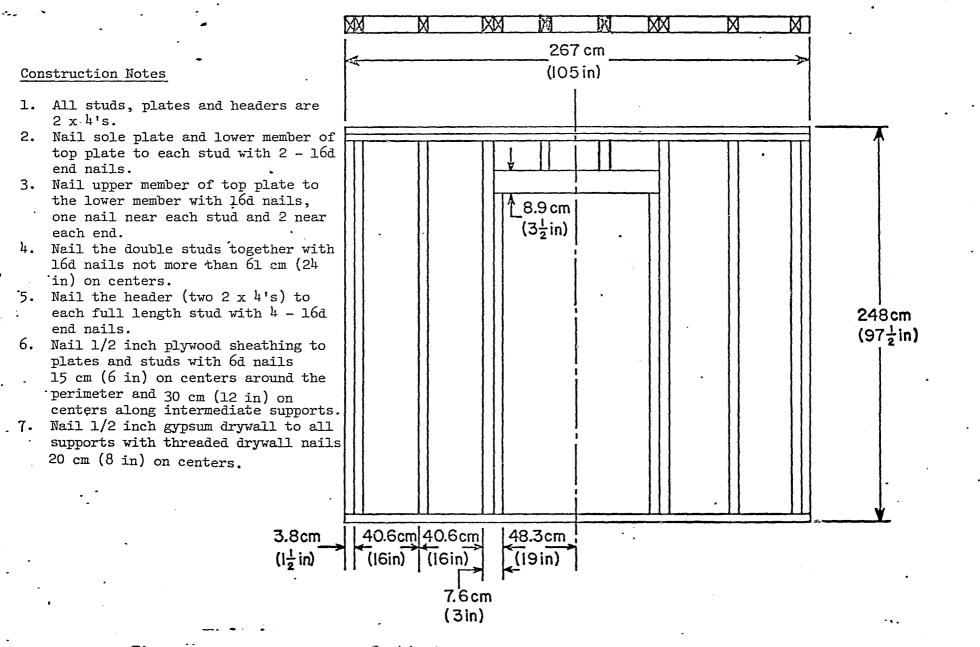
Figure 2. Door, Door Jamb, Hinge, and Lock Strike Component Fixture
