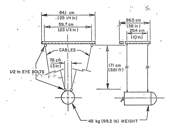
Figure B-3. Door Ram Suspension System
