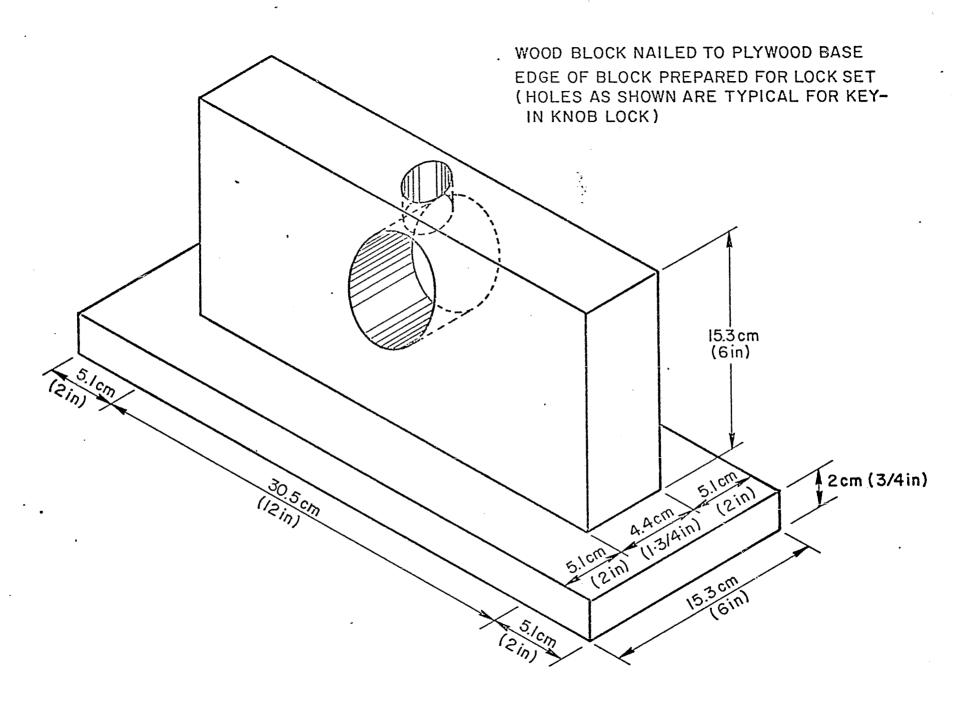
Figure 4: BOLT PRESSURE TEST FIXTURE
