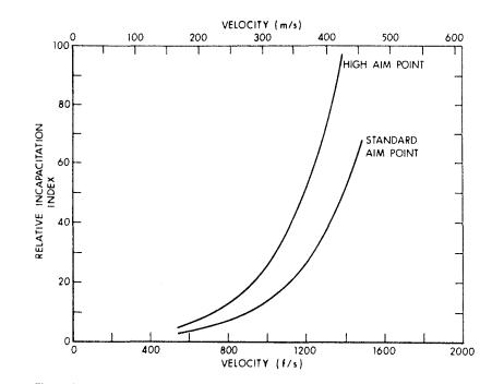
Figure 5. Effect of aim point on relative incapacitation index for group A officers at a range of 6 meters.
