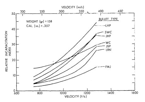
Figure 2. Relative Incapacitation Index as a function of velocity for seven bullet types in caliber ,357 (.38 Special). Each curve represents the average performance for all brands of the given bullet type. Differences among manufacturers can be distinguished, and will be reported in the final report.
