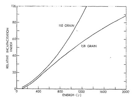
Figure 1. A comparison of a light bullet with a heavier bullet. Note the different values of relative incapacitation index at equal values of striking energy. Each are caliber .357 (.38 Spec.) semi-jacketed hollow points.
