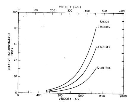
Figure 4. Effect of engagement range on relative incapacitation index for 125 grain semi-jacketed hollow point caliber .357 (.38 Spec.) bullets.
