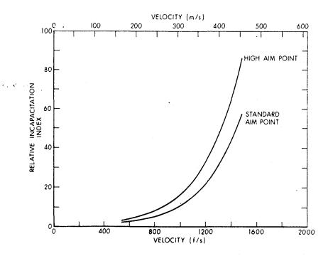
Figure 6. Effect of aim point on relative incapacitation index for group B officers at a range of 6 meters.
