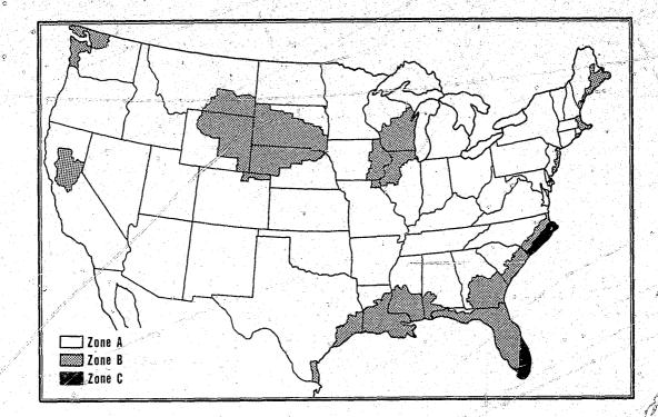
Figure 1. Location of wind loading zones based on 50 year mean recurrence interval.
