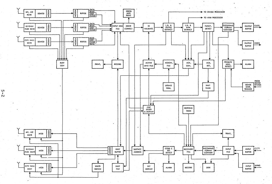
Fig. 4. Base Station Terminal Control Unit Block Diagram
