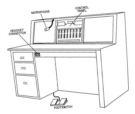
Figure 25. Standard production console unit.
