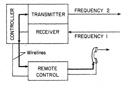
Figure 44. Base station/repeater receive-repeat mode.
