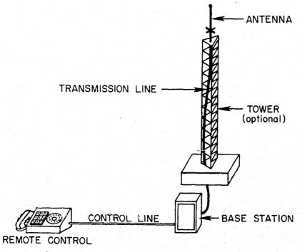
Figure 21. Base station-remote operation.
