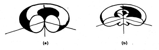
Figure 22. Three dimensional sketch of the radiation patterns of (a) a dipole antenna, (b) an antenna with directivity gain.
