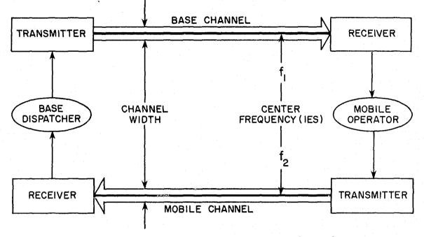
NOTE:  $f_1$  and  $f_2$  are the same for a single-frequency channel
