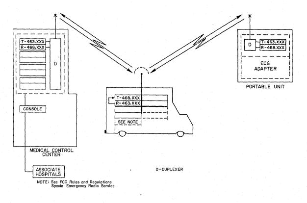
Figure 49a. UHF vehicular repeater concept (simplex one-way repeater).
