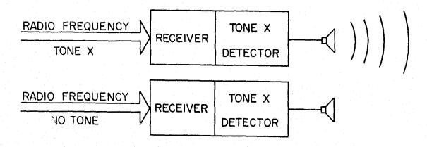
Figure 51. Continuous tone-coded squelch.
