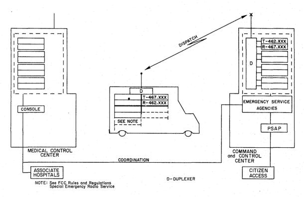
Figure 48a. UHF command and control (full duplex).
