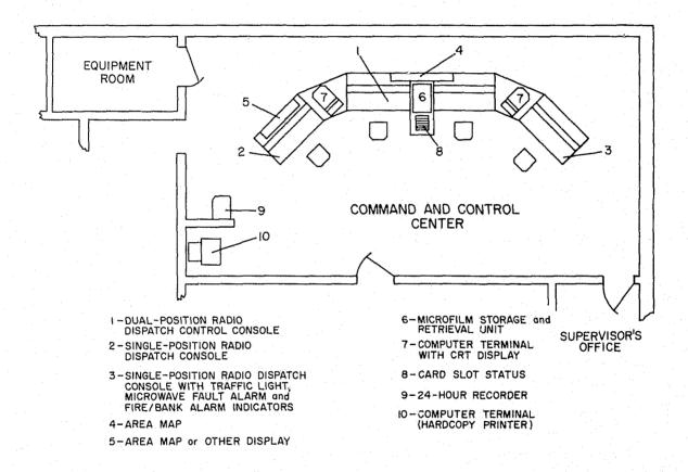
Figure 39. Typical medium-sized communication center.
