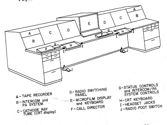
Figure 26. Special control console unit.
