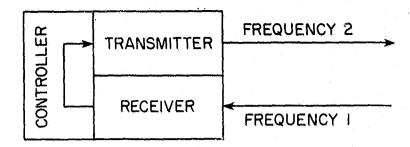
Figure 43. Duplexed radio station information relay.
