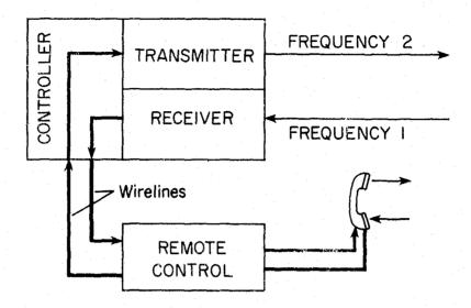
Figure 45. Base station/repeater transmit mode.
