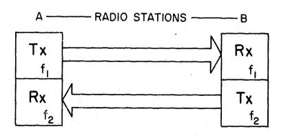
Both Stations A and B can transmit simultaneously on two frequencies
