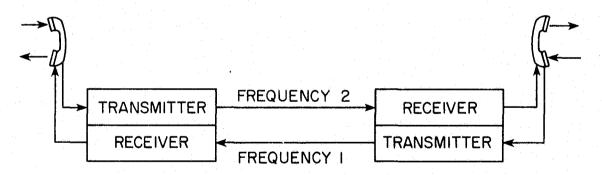
Figure 42. "Full duplexed" radio system simultaneous information exchange.
