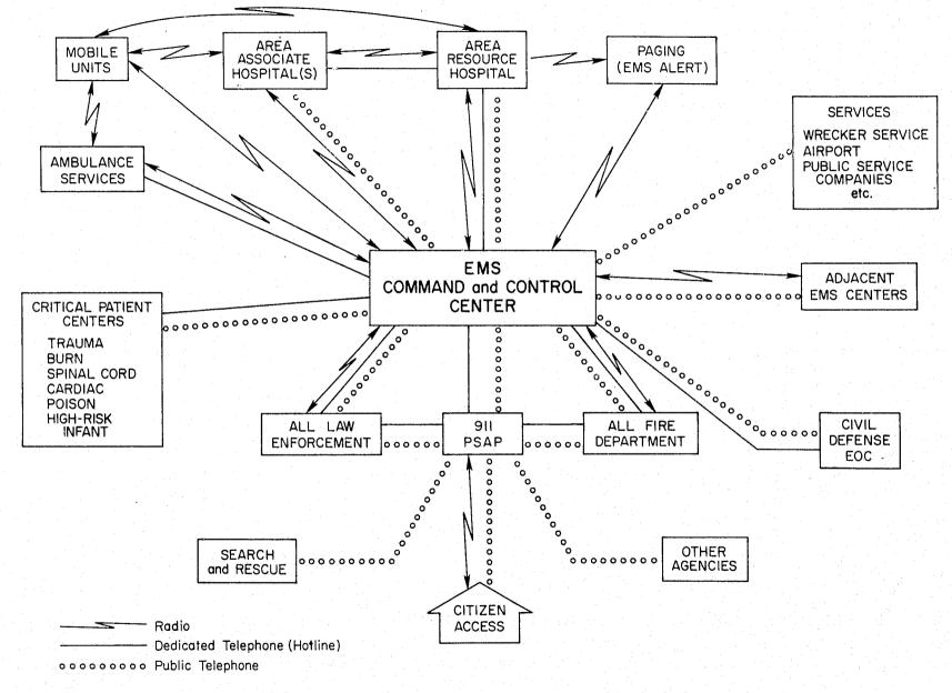
Figure 38. Typical system telephone and radio links.
