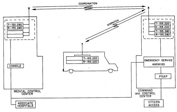
Figure 46a. VHF command and control (simplex).
