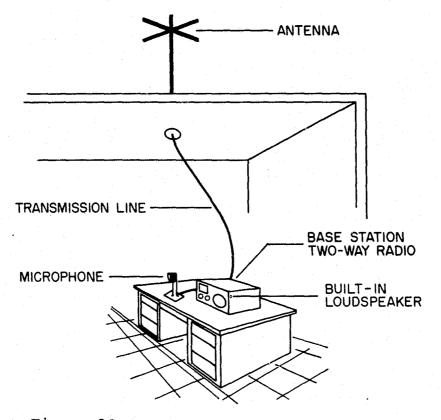
Figure 20. Typical small base station.
