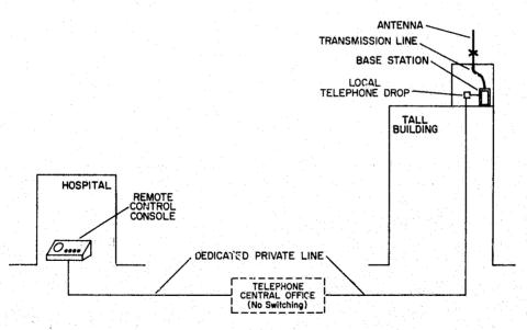
Figure 28. Remote control utilizing leased dedicated telephone line.
