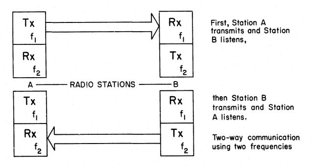
Figure 17. Two-frequency, simplex operation--permitting transmission from A to B or from B to A on two distinct frequencies, but not in both directions simultaneously.
