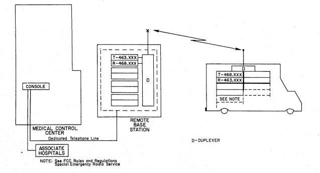
Figure 50b. UHF remote base station (full duplex).
