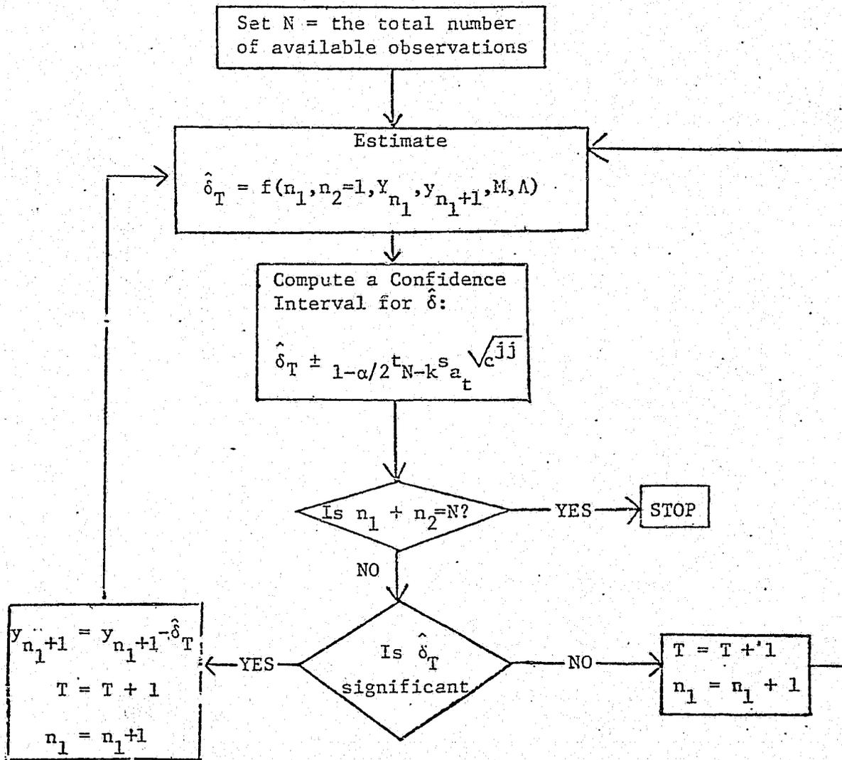
Figure 3. Flowchart for Identification Algorithm
