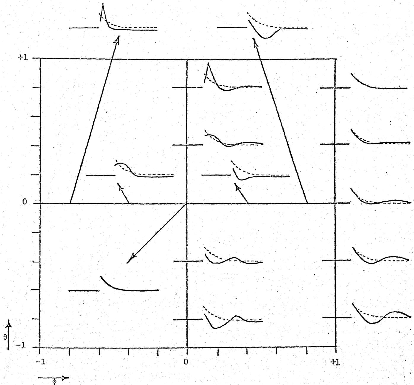
Figure 7. Effect of Variables  $M$  and  $A$  ( $\phi$  and  $\theta$ ) on the Decaying Pulse Response Model
