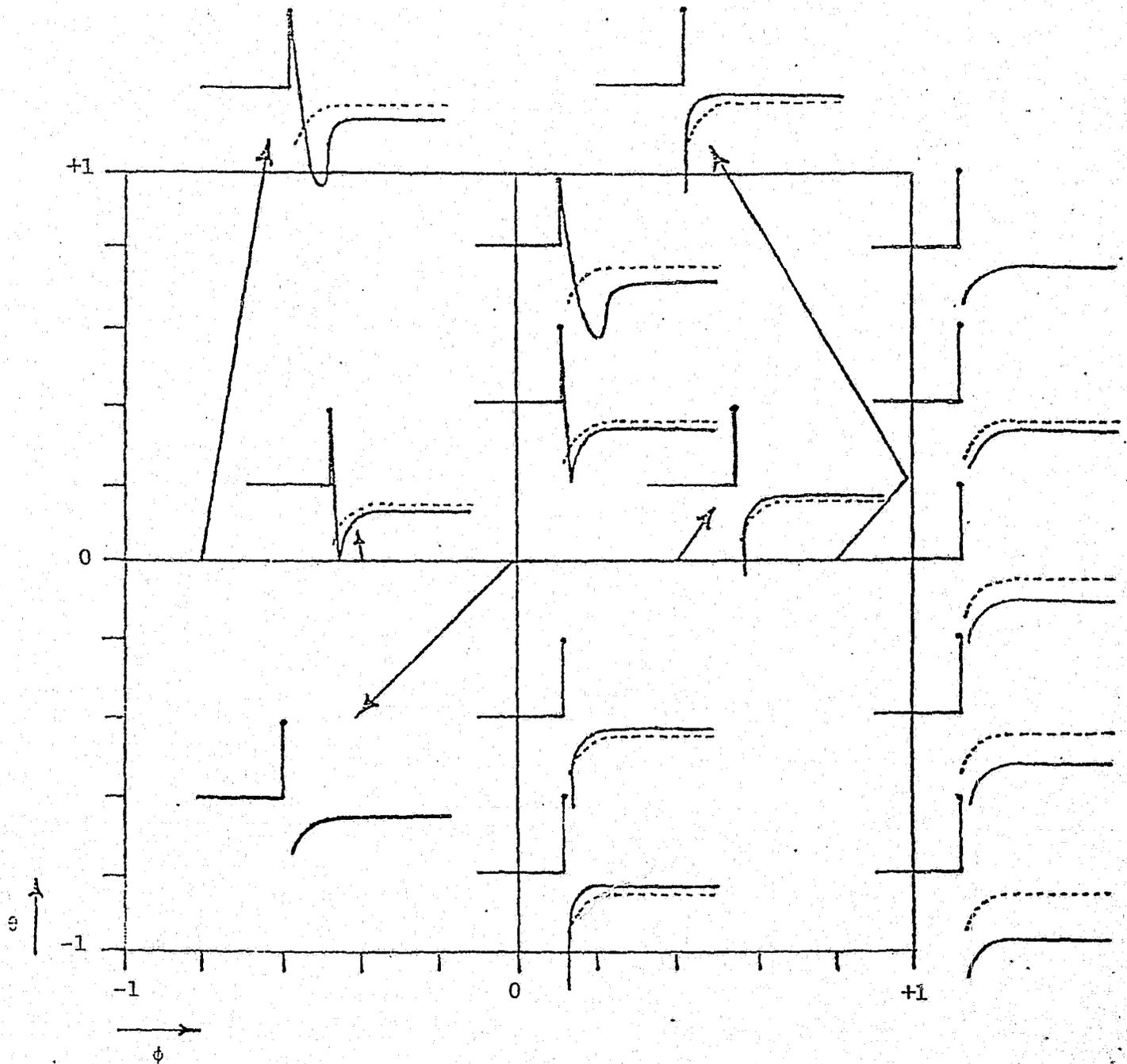
Figure 9. Effect of Variables M and  $\Lambda$  ( $\phi$  and  $\theta$ ) on the Inverse Decaying Pulse Response Model
