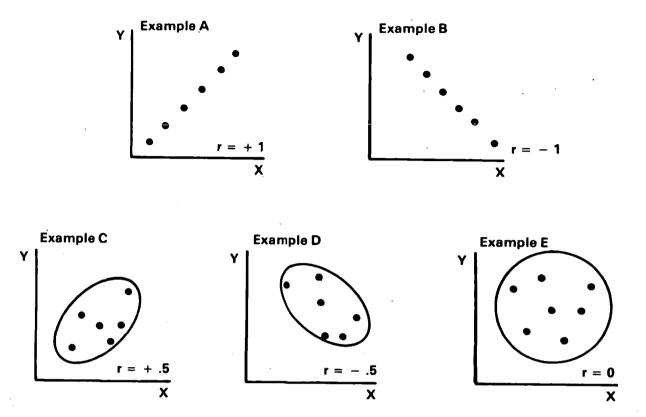
The direction of a correlation (positive or negative) can be seen instantly by whether the scattergram slopes up (Examples A and C) or down (Examples B and D) from left to right. The fatter the scatter (Example E) the smaller the r, the extremes being r = 1 (then the scattered points fall exactly on a straight line) and when r is 0.8
