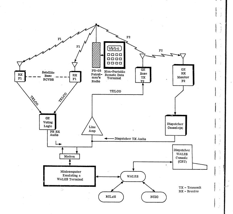
Figure 4-3. Digital System Layout
