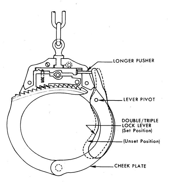
Figure 6. Partial cross section of improved handcuff with the double lock bolt inactive.
