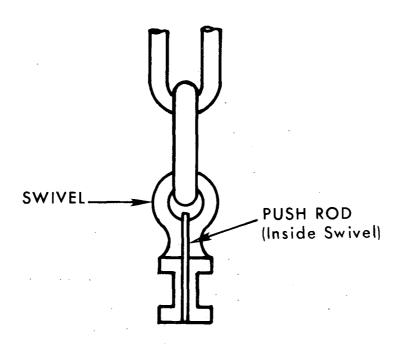
Figure 5. Alternate method of unseating an active double lock bolt.
