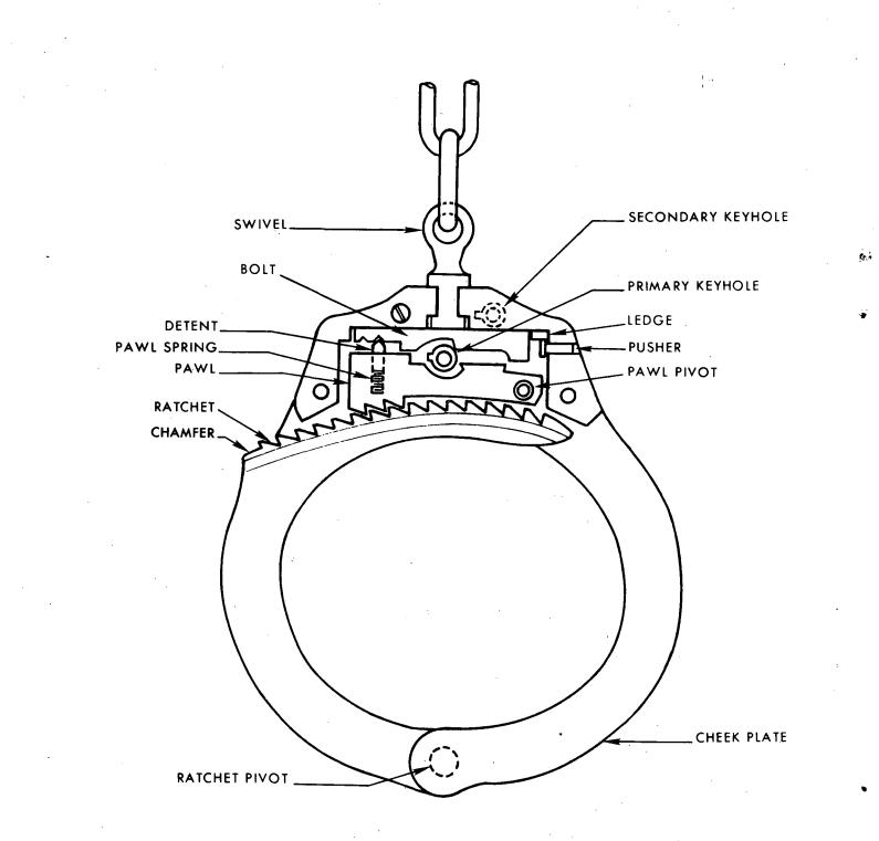
Figure 4. Partial cross section of a modified handcuff showing the secondary keyhold for unseating the double lock bolt and the chamfer of the last tooth of rachet.
