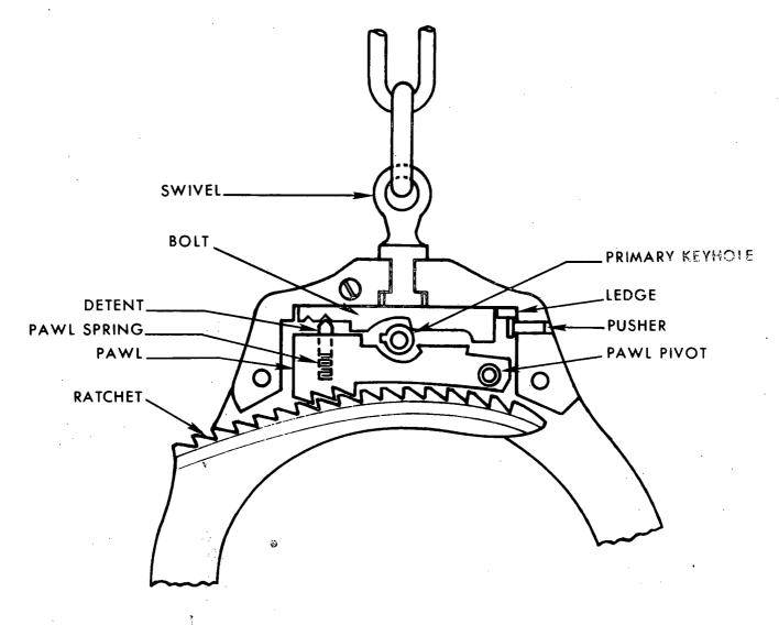
Figure 3. Cross section of a modified handcuff with the double lock bolt active and held in place by a locking ledge.
