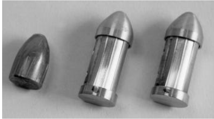
Figure 2. ATF master bullet No.1 obtained by a standardized shooting procedure (left) and NIST prototype standard bullets No.1 and 2 made by NC diamond turning process (middle and right)
