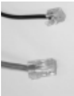
RJ45 LAN Cable & RJ11 Phone Cable
