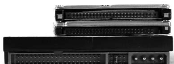
IDE power and data connections
