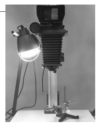
**Direct Lighting.** Direct lighting provides strong lighting from a source without the light first having been reflected off another surface. This type of lighting produces substantial contrast between the light and dark areas of the object being photographed. Direct lighting is set up with two or four lights equally balanced and set 45 degrees above the object, with the light shining directly onto the object (Figure 8-8).
