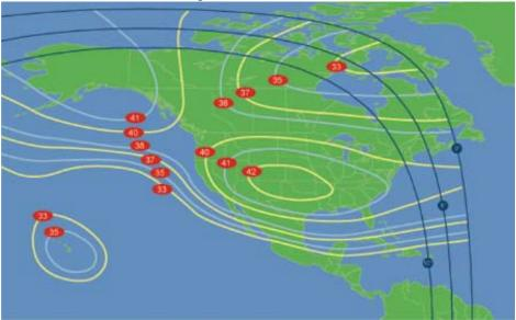
e. AMC-8/Aurora III, 139 degrees. This satellite jointly owned by SES and ATT was specifically designed to provide enhanced C-band service to Alaska. AMC-8 coverage of Alaska is shown below. This does not show the special coverage of Alaska provided by the Aurora III transponders.
