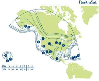
HORIZON 1 Horizontal Beam: Ku-Band EIRP Levels
