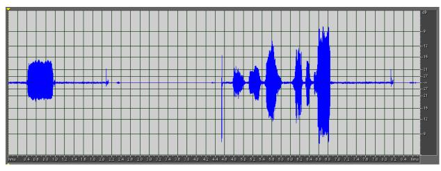
Figure 16 TYPICAL INTERFERENCE LIMITED AUDIO.GIF
