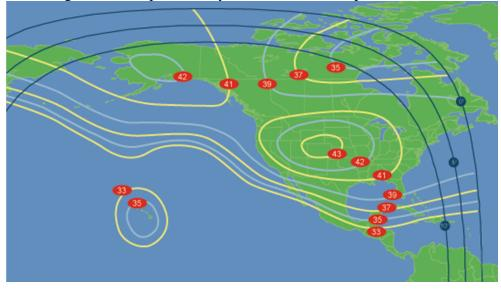
f. AMC-23. 172 degrees east longitude. This satellite is scheduled to be launched in November 2005 specifically to provide service to Boeing Connexcion (<u>www.boeingconnexcion.com</u>). Boeing Connexcion offers broadband IP service to aircraft and ships in the Pacific Ocean Area. Ku band
