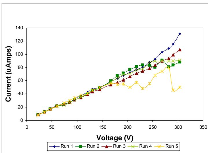
**Figure 7:** Ohm's law plot with flow of 1X TE buffer, using the eSPE device.
