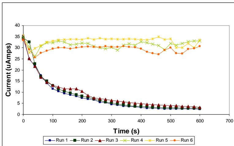
**Figure 5:** Results of buffer depletion experiments with and without flow of 1X TE with the electrodes in positions 1 and 2. Note that the current remains constant when flow is applied.
