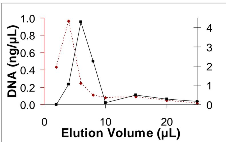
**Figure 2:** The elution of DNA from a silica-based micro solid-phase extraction ( $\mu$ SPE). The DNA, as determined fluorescently (red trace) elutes in approximately 10  $\mu$ L. PCR amplification, however, is only possible with the latter 6-8  $\mu$ L, a result of contaminating isopropanol from the protein removal step of the extraction.
