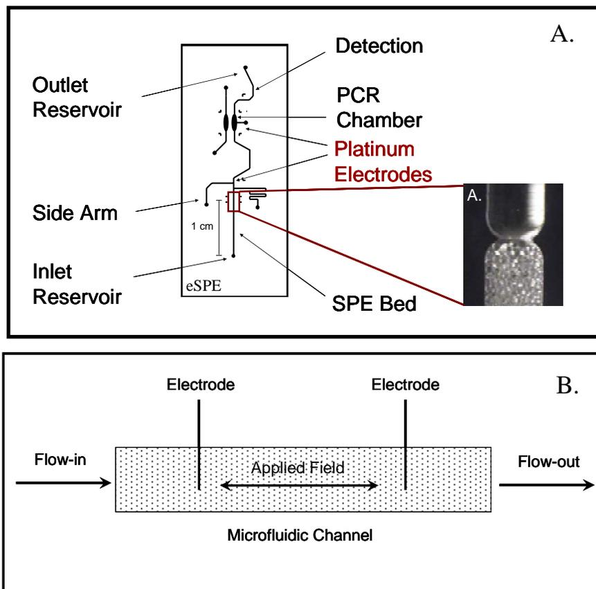
**Figure 1:** (A) The eSPE device design. Electrodes adjacent to the PCR chamber and just downstream of the SPE bed allow for application of field during the elution phase of the DNA extraction to concentrate eluting DNA. The side arm enables the addition of PCR reagents for future integration of PCR amplification. (B) Side view schematic of the microfluidic channel with inserted electrodes, allowing both flow and field mobilization of DNA to occur simultaneously.
