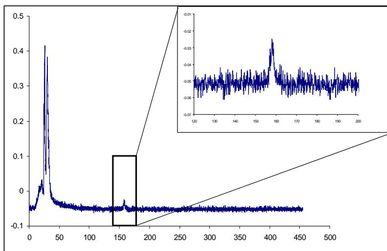
**Figure 12:** eSPE of fluorescein-labelled DNA. Note the presence of a large elution of DNA that passes through the field unperturbed; however a small amount of DNA (inset) is retained and eluted during the release phase.
