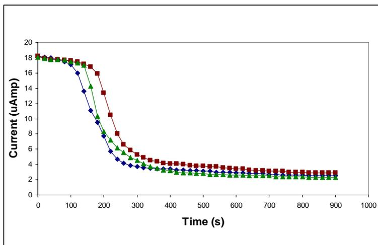
**Figure 4:** Buffer depletion experiments accomplished with (B) and without (A) flow of 1X TE buffer through the device. Note that although there is a slightly longer (approximately 50 s) before the severe drop in current is noted, the drop (indicative of buffer depletion) still occurs rapidly after application of field.
