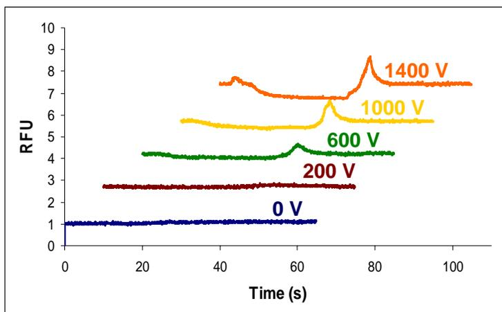
At field strengths higher than 1400 V/cm, Joule heating and bubble formation become
