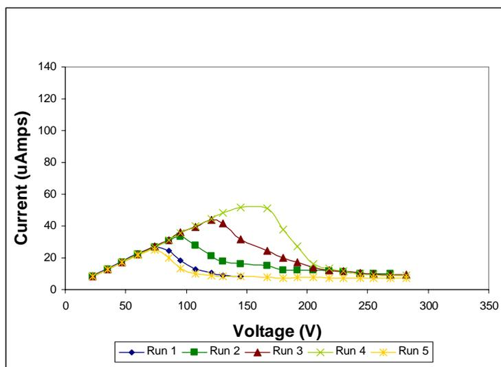
**Figure 6:** Ohm's law plot without flow of 1X TE, using the eSPE device.
