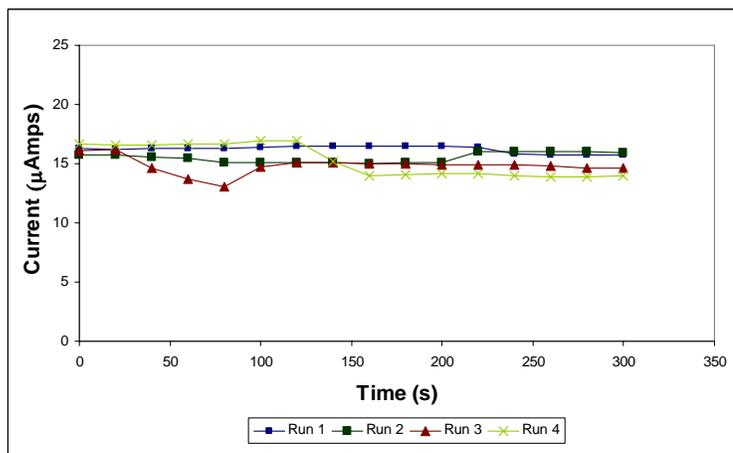
**Figure 8:** Consistent current was measured with Tris buffer and the applied voltage (1400 V) for up to 300 s (5 minutes), with no evidence of buffer depletion effects that could prove deleterious to DNA retention.
