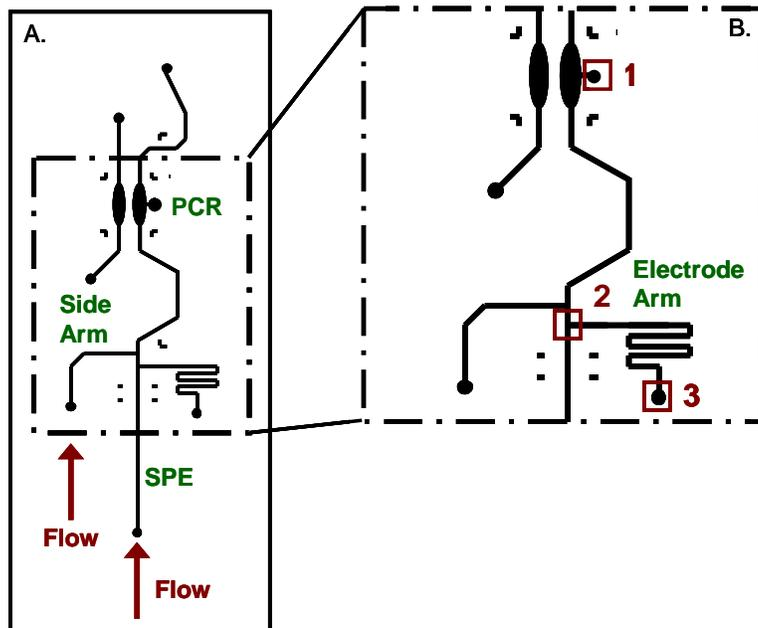
**Figure 3:** The eSPE device design showing solution flow (A) and electrode placement, numbered 1-3 (B). Electrodes are placed in position 1 and in position 2 or 3, as indicated for each experiment.
