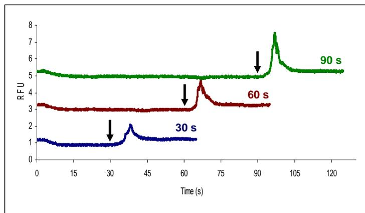
**Figure 11:** Precision retention and release of DNA from the eSPE device. Field was applied for varying lengths of time as indicated (arrows indicate where field is reversed for 5 s, followed by termination of field), while DNA (5 ng/ $\mu$ L) was flowed continuously at 250  $\mu$ L/hr through the device. DNA eluted past the detector only when the reverse field release step occurred
