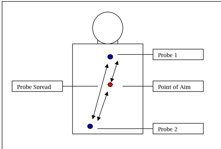
In addition to the simple measures of probe spread and distance from point of aim, additional data points were captured as “Distance to Miss.” This variable is indicative of a measure of how close the probe came to missing the target. This variable was constructed in order to capture an additional dimension of accuracy and the likelihood of a failed
