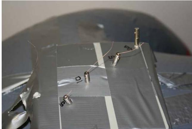
**TASER:** At the 5-foot distance interval the TASER probe and barb penetrated completely past the base of the probe. The base of the probe penetrated approximately 7/16 of an inch.
