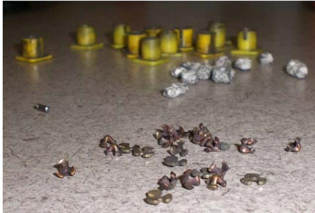
Further problems existed in that the Stinger cartridges would also discharge little pieces of plastic and metal that could best be described as “shrapnel”. This was noted numerous times in testing as these items constantly struck the research team. These items were randomly dispersed and would sometimes fly out at nearly a 90-degree angle to the weapon, striking people next to the person deploying the Stinger S200.
