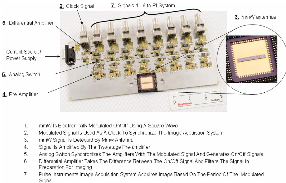
**Figure 8. Proto-type Board.** 8-channel proto-type built COTS parts to acquire and amplify detector signals.
