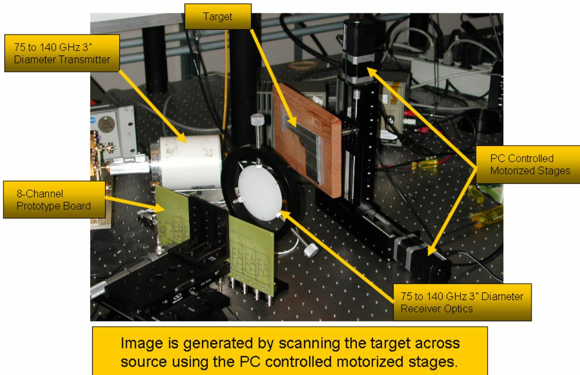
**Figure 9. mmW Test Set-up.** 8-channel mmW proto-type board integrated onto the Zaber stages in preparation for image generation.
