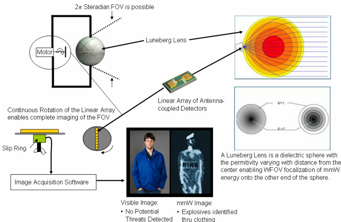
**Figure 4. mmW Imaging.** A linear detector continuously rotated enables complete imaging of the FOV captured by the luneberg lens.
