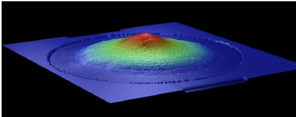
**Figure 3. Micro-lens Development.** Resist profile measured with a Veeco optical profiler showing the potential for development of a micro-lens using a gray-scale mask.
