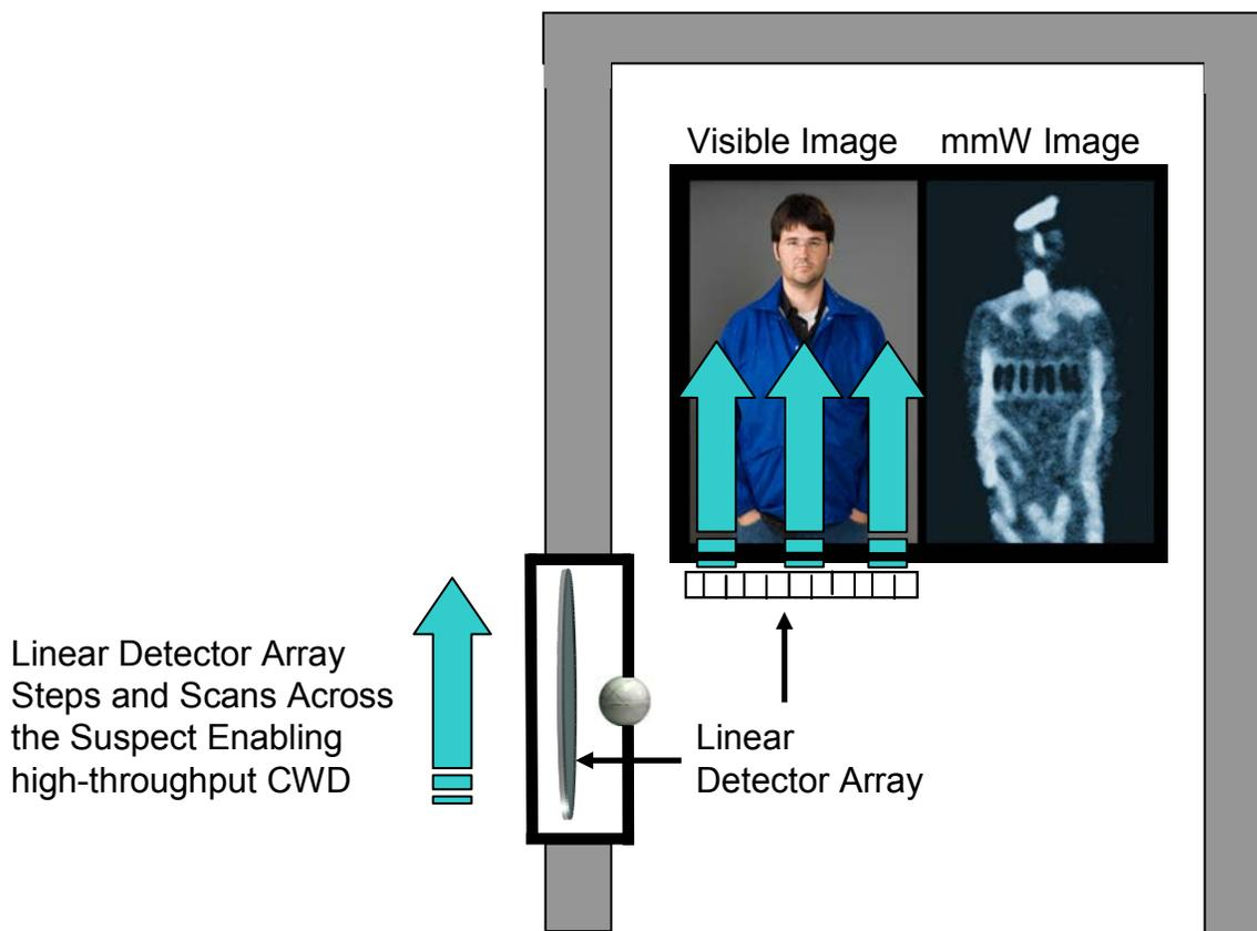
**Figure 5. Alternate Approach for a High-throughput CWD Imaging Portal by Stepping and Scanning the Linear Detector Array Across the Suspect.**
