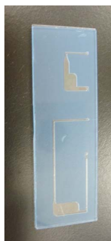
Figure 13. (left) Flow cell. PCR chamber on the bottom and APEX chamber on the top. (right) APEX allele signal ratio results obtained for an eye color SNP at position RS1800407. PCR was performed in the flow cell positioned in the bladder thermal cycler. Flow cell results were compared to a positive control (0.2 ml PCR tube) amplified in an MJ thermal cycler and a Cepheid tube also positioned in the bladder thermal cycler. APEX was performed offline for one hour. Results indicate comparable APEX signals for all three PCR approaches and confirm the homozygous GG genotype.
