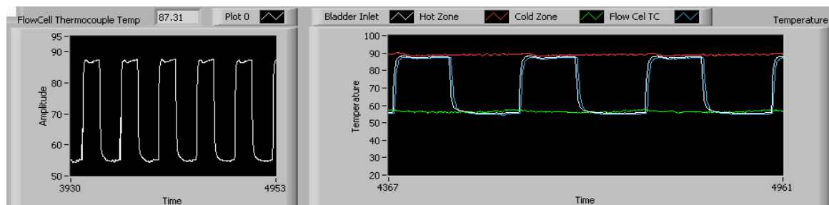
Figure 29. Thermal cycling profile with PID pump and heater control. Red line shows the temperature of the hot zone, green line shows the cold zone, the white line shows the temperature of a thermocouple sandwiched between the bladders, and the blue line shows the temperature of the working fluid just prior to entering the bladder.
